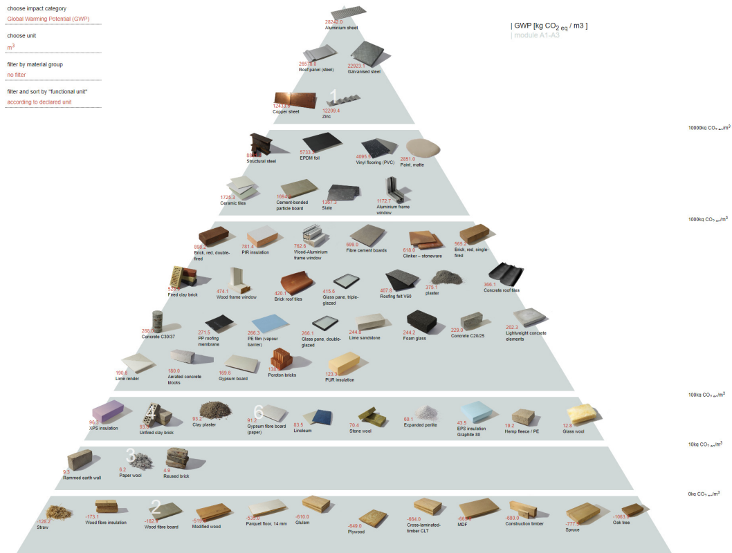
Figure 4.1: Building Material Pyramid retrieved from [79]
