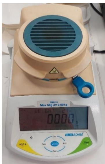
Figure 15. PMB 53 moisture analyser (ADAM, UK).
