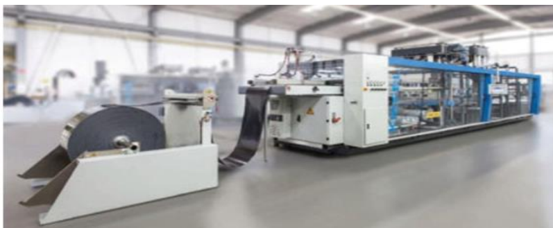
Figure 1. One example of roll-fed thermoforming machine (Spalding & Chatterjee 2017, p. 586).
