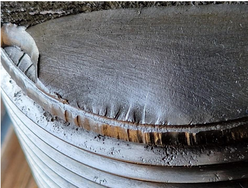
Figure 22. Main fatigue crack at the first fully formed thread with visible ratchet marks.
