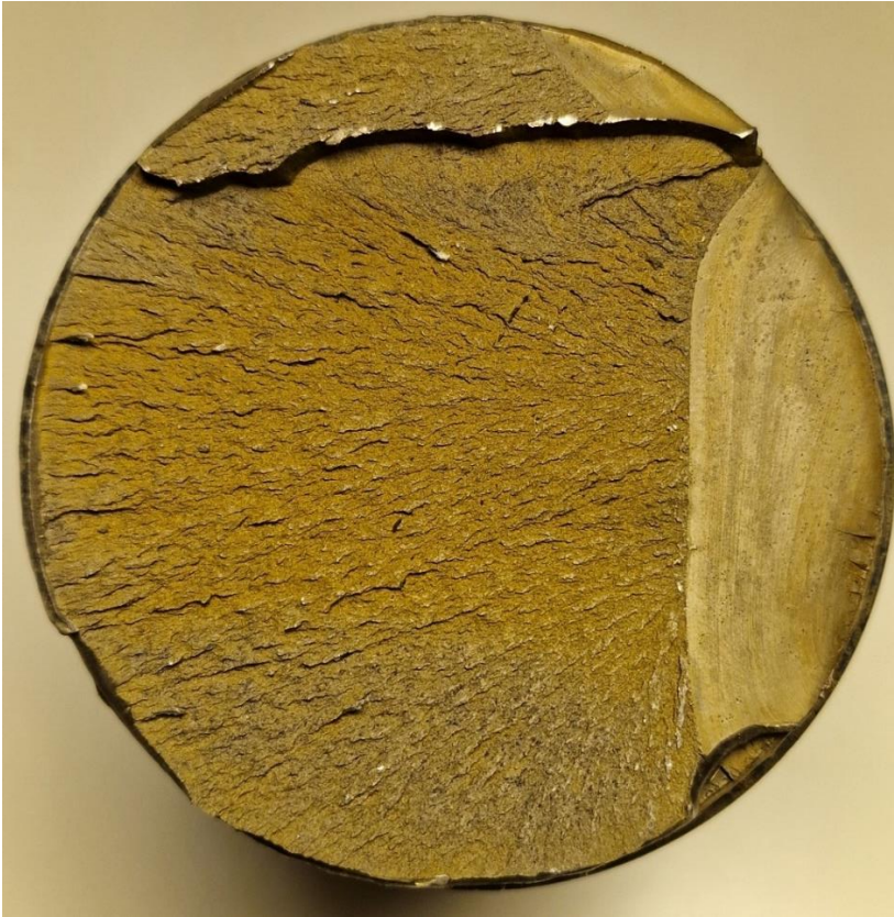
Figure 21. Broken bolt showing signs of propagating fatigue cracks in two separate locations.
