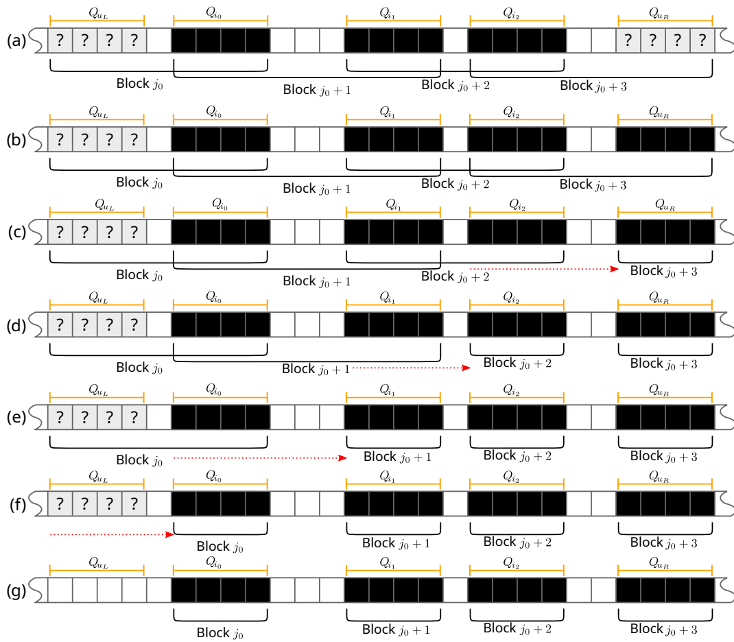
Figure 32. Shows an example of edge mix. (a) is state of relevant line segment initially, (b) is colouring of Q_{u_R} to black, (c) to (f) are chaining block's range reductions, and (g) .
