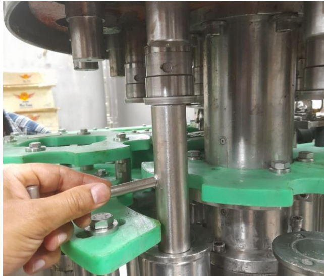
Figure 32. Measuring the pin height.
