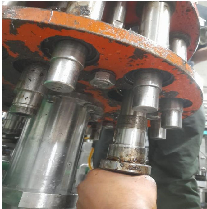
Figure 33. Disassembling the chuck shaft from seamer.
