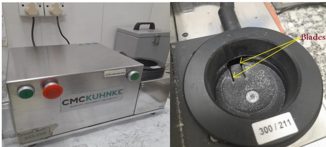
Figure 16. Cutter device for sectioning of cans.
