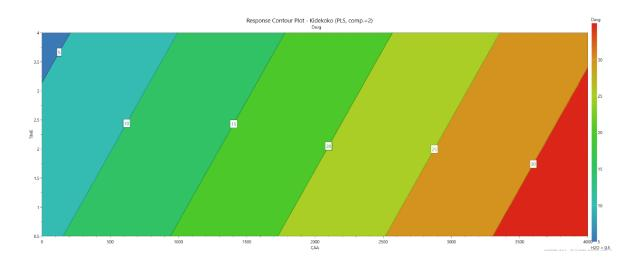
Figure 64 Responsive contour plot for particle size. The mixing time (min) on the yaxis and the amount of CA (ppm) on the x-axis. The largest particle size could be achieved with a moderate mixing time when the amount of CA is to maximum.
