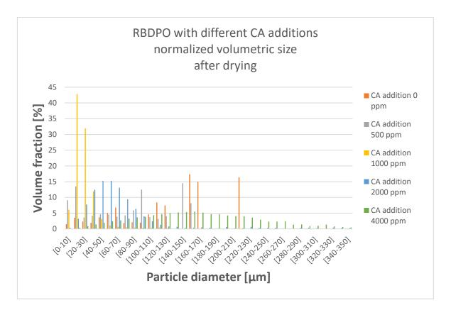
Figure 30 RBDPO with different CA additions, normalized volumetric size data obtained from Pixact measurement. Data from the samples after the drying procedure.
