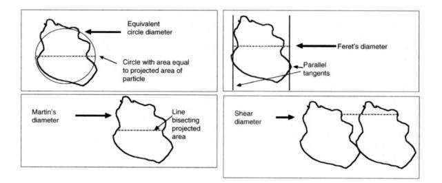
Figure 12 Different particle diameters presented by Rhodes (2008)
