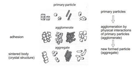
Figure 16 Relationship between individual particles, agglomerates and aggregates. (Walter, 2013)
