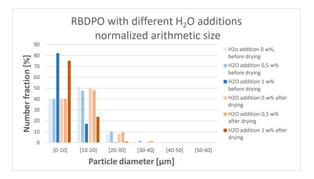
Figure 39 RBDPO with different water additions, normalized arithmetic size data obtained from Pixact measurement. Data from the samples before and after the drying procedure.
