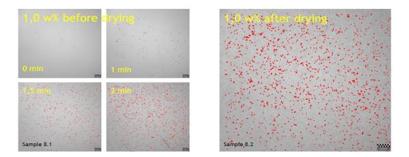
Figure 33 Exp 8, on the left there is the sample after acid treatment and on the right after drying. Feedstock in the experiment is RBDPO and the water addition is 1.0 w%.
