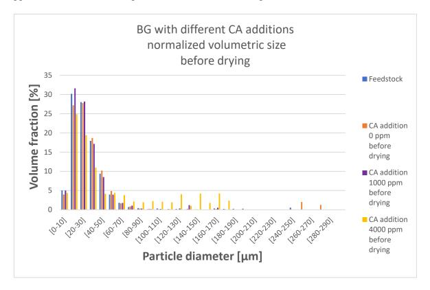
Figure 103 The volumetric size distribution of BG samples, with different CA additions.
