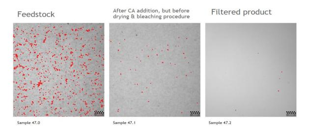
Figure 101 exp 47. Technical feedstock, CA addition 4000 ppm. Feedstock on the left side, product after acid treatment in the middle, filtered product on the right
