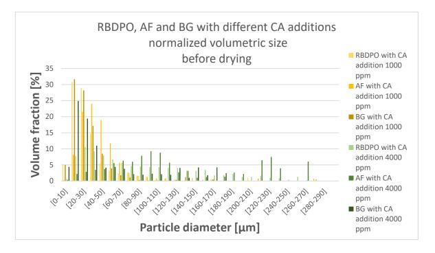
Figure 106 The normalized volumetric size distribution for the samples of different feedstocks containing 1000 ppm or 4000 ppm of CA. The analysis has been performed before filtration.
