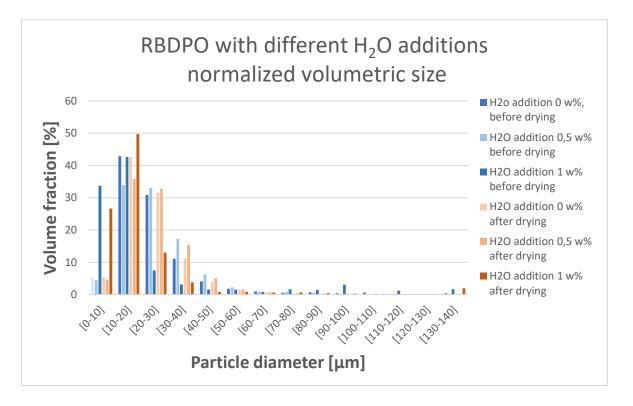
Figure 40 RBDPO with different water additions, normalized volumetric size data obtained from Pixact measurement. Data from the samples before and after the drying procedure.
