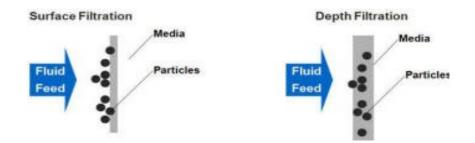
Figure 9 the principle of surface filtration is presented on the left, and the principle of depth filtration on the right. (FDPP)
