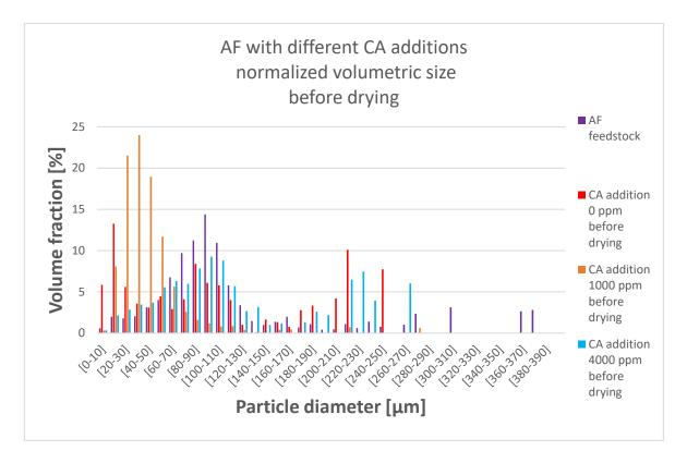
Figure 98 The normalized volumetric size distribution for AF samples with different CA additions
