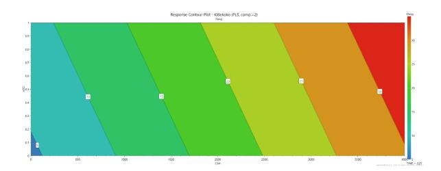
Figure 63 Responsive contour plot for particle size. The amount of water (w %) on the y-axis and the amount of CA (ppm) on the x-axis. The size of the particles can be indicated to increase when increasing the concentration of CA and the amount of water. The largest particle size could be achieved with a large water and CA additions.
