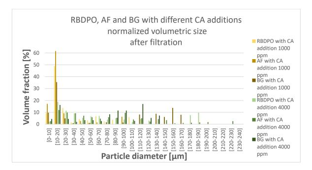
Figure 107 The normalized volumetric size distribution for the samples of different feedstocks containing 1000 ppm or 4000 ppm of CA. The analysis has been performed after filtration.
