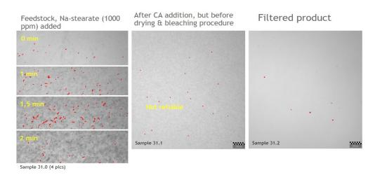
Figure 84 exp 31. Sodium stearate addition of 0,002 mol, CA addition 1000 ppm. Feedstock on the left side, product after acid treatment in the middle, filtered product on the right.
