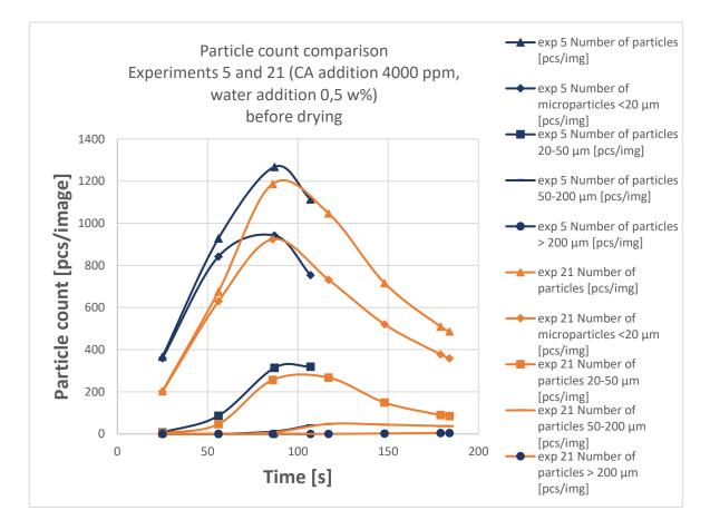
Figure 73 The particle count comparison for experiments 5 and 21, where the feedstock is RBDPO and the CA addition 4000 ppm.
