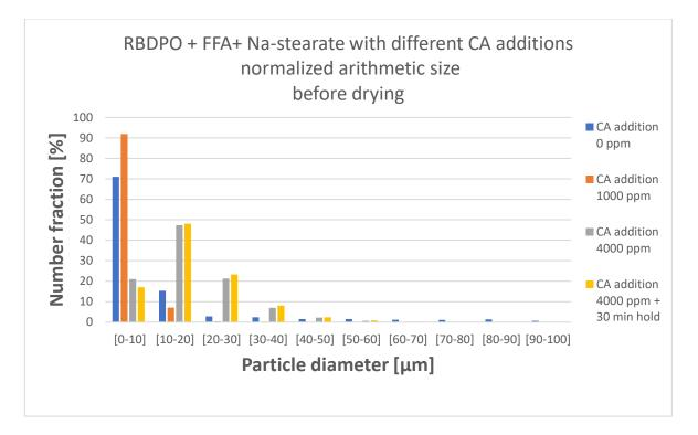
Figure 86 Normalized arithmetic size distribution with the samples containing RBDPO, FFA and Na-stearate. Samples have different CA additions, and they are measured before the drying procedure.
