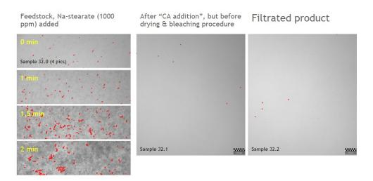
Figure 83 exp 32. Sodium stearate addition of 0,002 mol, CA addition 0 ppm. Feedstock on the left side, product after acid treatment in the middle, filtered product on the right.
