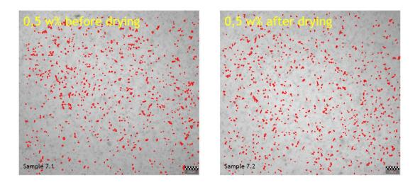
Figure 32 Exp 7, on the left there is the sample after acid treatment and on the right after drying. Feedstock in the experiment is RBDPO and the water addition 0.5 w%.
