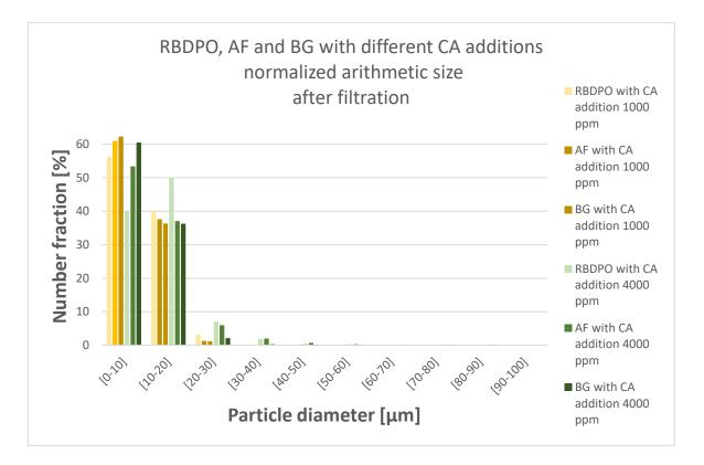
Figure 105 The normalized arithmetic size distribution for the samples of different feedstocks containing 1000 ppm or 4000 ppm of CA. The analysis has been performed after filtration.
