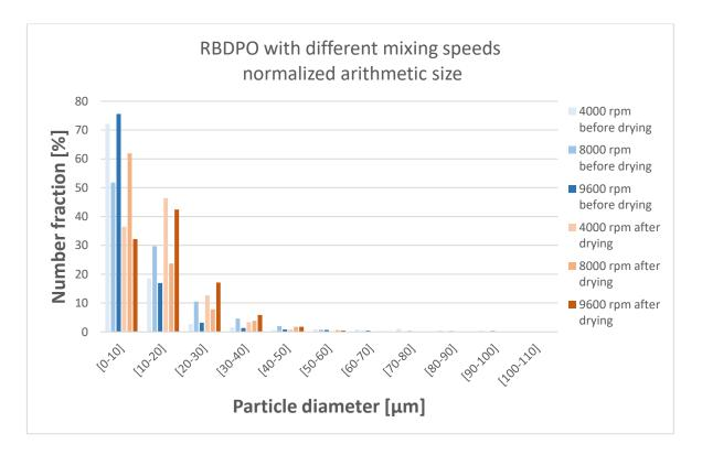
Figure 51 Different mixing speed comparison for RBDPO samples with 1000 ppm of CA and 0.5 w% of water. Larger particles are present in the samples after drying.
