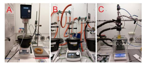
Figure 17 A) High shear mixer with oil bath and the vessel, B) Three-neck flask in the oil bath for bleaching, C) batch filtration equipment
