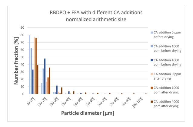
Figure 75 Normalized arithmetic size distribution for the experiments with FFA in the feedstock. The CA addition varies in these samples.
