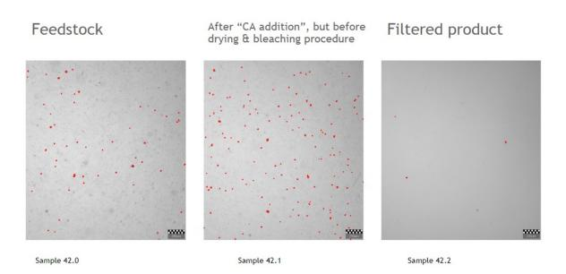
Figure 94 exp 42. Technical feedstock, CA addition 0 ppm. Feedstock on the left side, product after acid treatment in the middle, filtered product on the right.
