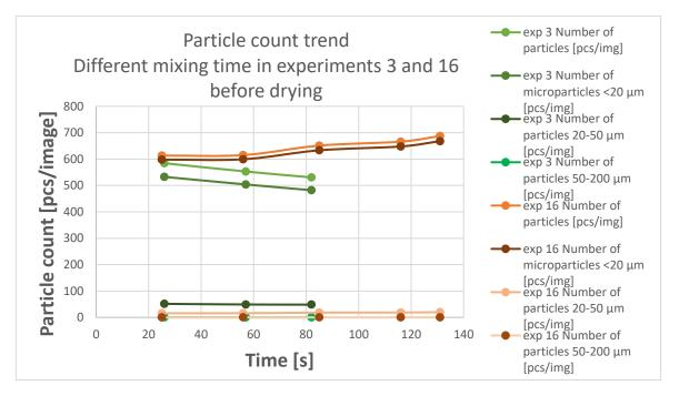
Figure 49 Particle count trend from the experiments 3 and 16. The mixing time in exp 3 was 2 minutes, and in exp 16 4 minutes.
