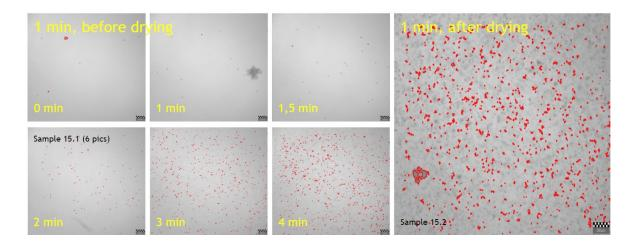
Figure 47 Exp 15, on the left there is the sample after acid treatment and on the right after drying. Feedstock in the experiment is RBDPO and the high shear mixer condition used in this experiment was 8000 rpm for 1 minute.
