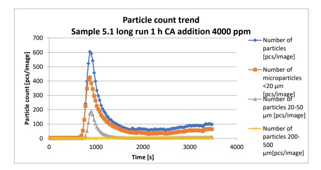
Figure 16 Particle count during the Pixact measurement. The number of counted particles (from 0 µm to 400 µm max) stabilized after 30 minutes.
