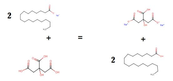
Figure 80 Reaction equation for sodium stearate and citric acid. One CA molecule can react with two Na-stearate molecules. There is a possibility for a third reaction, as the centre group remains unharmed.
