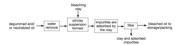
Figure 8 Bleaching process. The water removal is possible to perform before or after the bleaching earth/clay addition. (Silverson)
