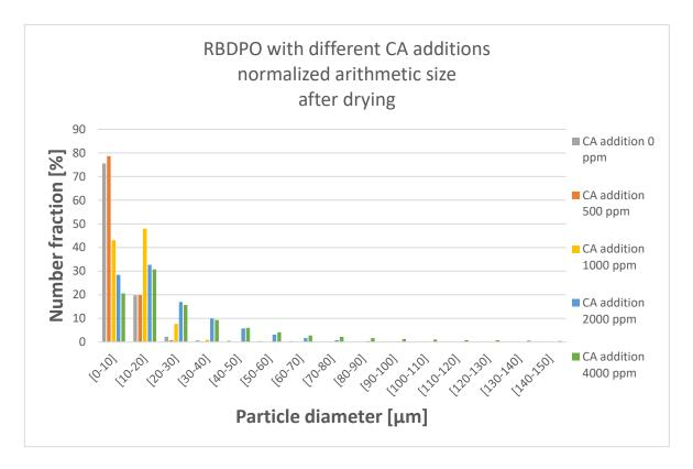
Figure 28 RBDPO with different CA additions, normalized arithmetic size data obtained from Pixact measurement. Data from the samples after the drying procedure.
