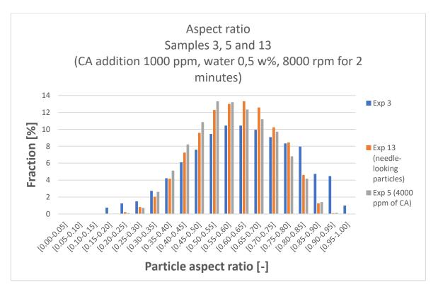
Figure 45 Aspect ratio from the experiments 3, 5 and 13. Exp 3 and 13 had similar conditions, but a bit different-looking particles. Exp 5 had a bigger amount of CA added to the solution.
