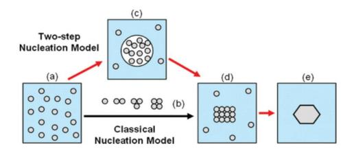
Figure 14 Crystal formation via different pathways: a) supersaturated solution b) classical nucleation theory, where the subcritical cluster of solute molecules are organised c) liquid-like cluster of solute molecules in denser or supersaturated environment d) ordered crystalline nuclei e) solid crystal (Erdemir et al, 2009)
