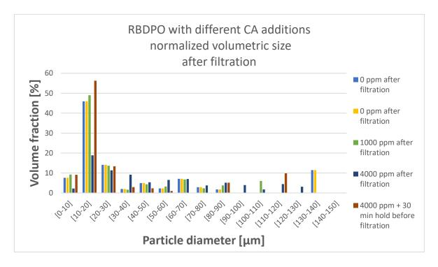
Figure 61 Normalized volumetric size distribution after filtration for the samples with different CA additions.
