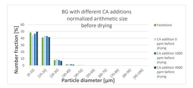
Figure 102 The normalized arithmetic size distribution of BG samples, with different CA additions.
