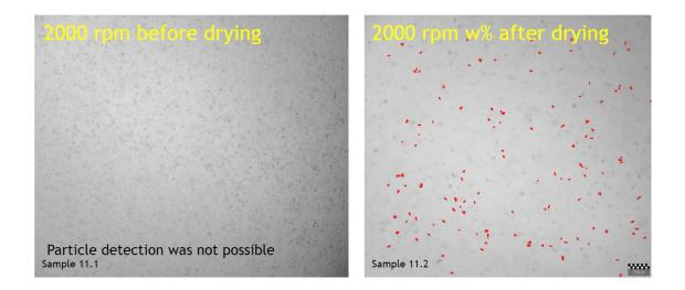
Figure 41 Exp 11, on the left there is the sample after acid treatment and on the right after drying. Feedstock in the experiment is RBDPO and the high shear mixer condition used in this experiment was 2000 rpm for 2 minutes.
