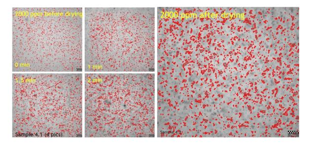
Figure 22 Exp 4, on the left is the sample after acid treatment (4 small pictures) and on the right after drying. Feedstock in the experiment is RBDPO and the CA addition is 2000 ppm.
