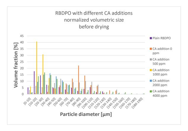
Figure 29 RBDPO with different CA additions, normalized volumetric size data obtained from Pixact measurement. Data from the samples before the drying procedure.
