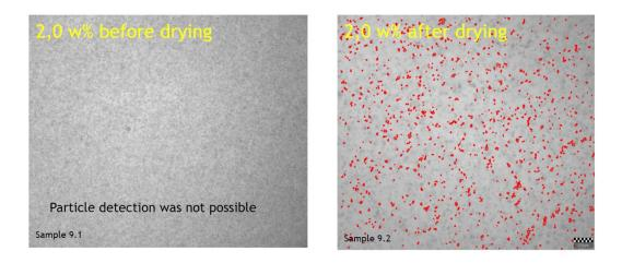
Figure 36 Exp 9, on the left there is the sample after acid treatment and on the right after drying. Feedstock in the experiment is RBDPO and the water addition 2.0 w%.
