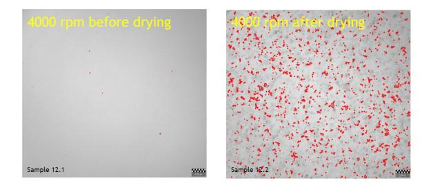
Figure 42 Exp 12, on the left there is the sample after acid treatment and on the right after drying. Feedstock in the experiment is RBDPO and the high shear mixer condition used in this experiment was 4000 rpm for 2 minutes.
