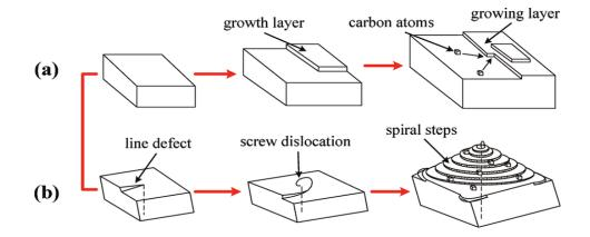
Figure 15 Possible growing routes for a crystal. A) Presents adsorption layer theory, and B) presents the screw dislocation in the growth. (Liu et al, 2011)
