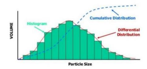
Figure 11 Different particle size distribution models presented by Treviranus (2011).
