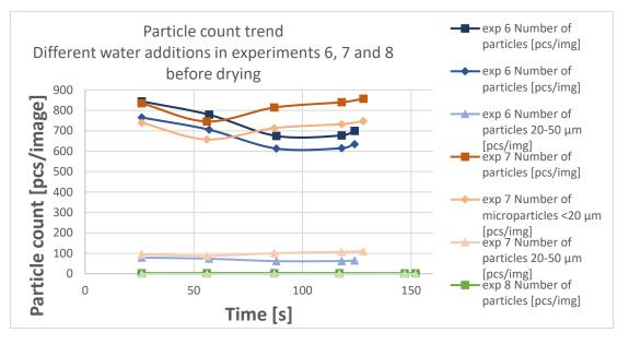
Figure 34 Particle count trends from the experiments 6, 7 and 8, with water additions 0, 0.5 and 1 w% respectively. Before the drying procedure.
