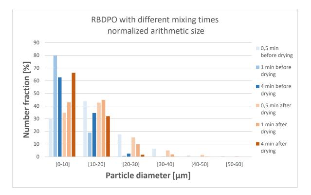
Figure 52 Different mixing time comparison for RBDPO samples with 1000 ppm of CA and 0.5 w% of water. Larger particles are present in the samples after drying.
