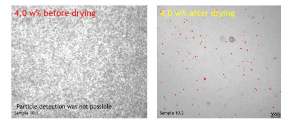
Figure 37 Exp 10, on the left there is the sample after acid treatment and on the right after drying. Feedstock in the experiment is RBDPO and the water addition is 4.0 w%.
