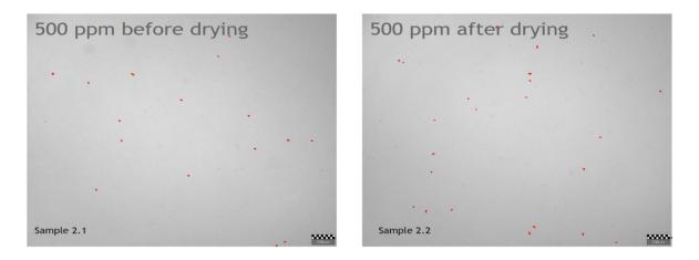
Figure 20 Exp 2, on the left there is the sample after acid treatment and on the right after drying. Feedstock in the experiment is RBDPO and the CA addition 500 ppm.
