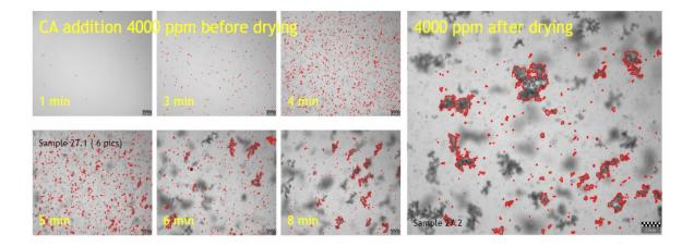
Figure 72 Exp 27, on the left there is the sample after acid treatment and on the right after drying. Feedstock is RBDPO+FFA and CA addition is 4000 ppm.
