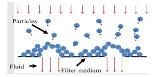
Figure 10 Bridging mechanism in filtration (Hund et al, 2017)
