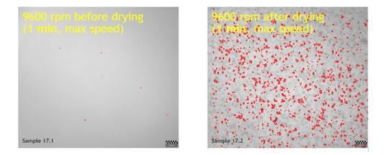
Figure 50 on the left there is the sample after acid treatment and on the right after drying. Feedstock in the experiment is RBDPO and the high shear mixer condition used in this experiment was 9600 rpm for 1 minute.
