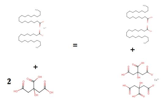
Figure 81 Reaction equation for calcium stearate and citric acid, one possible way. It is possible that the calcium ion bonds with two of three –OOH groups of CA molecule.
