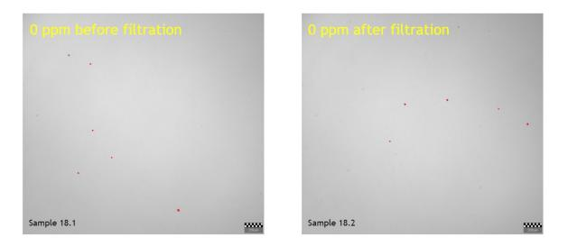
Figure 55 Exp 18, on the left there is the sample after acid treatment and on the right after filtration. Feedstock in the experiment is RBDPO and CA addition is 0 ppm.
