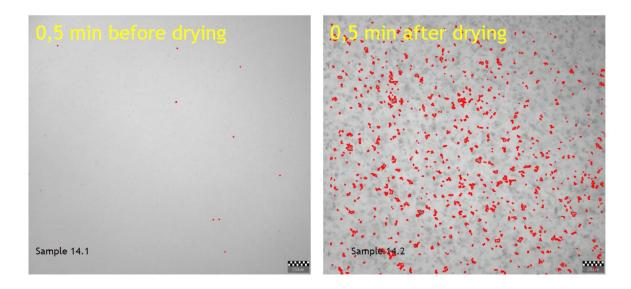
Figure 46 Exp 14, on the left there is the sample after acid treatment and on the right after drying. Feedstock in the experiment is RBDPO and the high shear mixer condition used in this experiment was 8000 rpm for 0.5 minutes.
