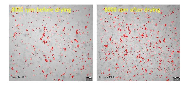
Figure 43 Exp 13, on the left there is the sample after acid treatment and on the right after drying. Feedstock in the experiment is RBDPO and the high shear mixer condition used in this experiment was 8000 rpm for 2 minutes.
