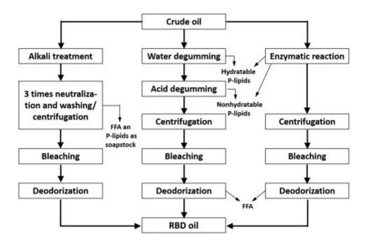
Figure 6 Possible pretreatment routes for crude bio-based oil. (Jiang, Y., 2019)
