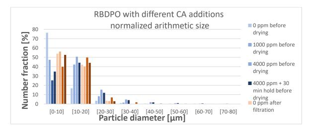
Figure 59 Normalized arithmetic size distribution for the samples with different CA additions before and after filtration. The size of the particles present in the solution remains the same before and after filtration. Please note that the Figure is showing percentages, not actual particle counts.
