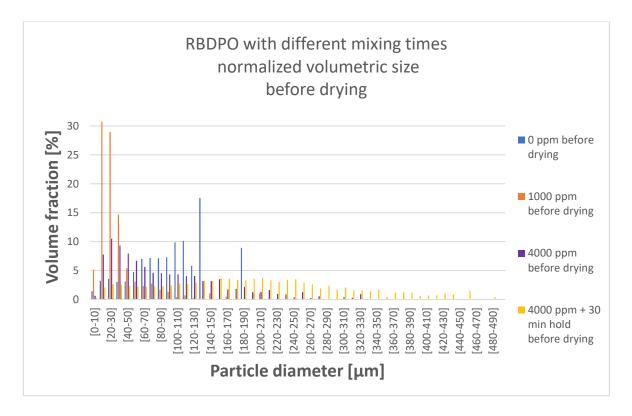
Figure 60 Normalized volumetric size distribution before drying procedure for the samples with different CA additions.
