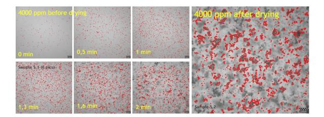
Figure 23 Exp 5, on the left is the sample after acid treatment (6 small pictures) and on the right after drying. Feedstock in the experiment is RBDPO and the CA addition is 4000 ppm.
