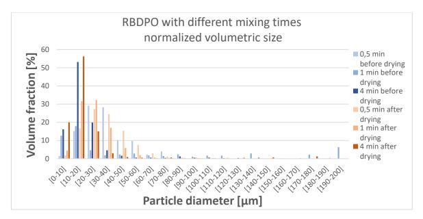
Figure 54 Volumetric size distribution for different mixing time comparison for RBDPO samples with 1000 ppm of CA and 0.5 w% of water. Volume of the particles seems to remain the same during the experiment.
