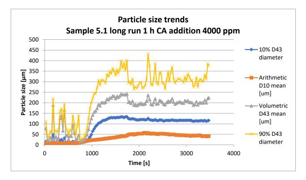
Figure 25 Increase of particle size from 0 to 50  $\mu$ m during 1 h measurement time in the Pixact measurement. The size of the particles seem to stabilize after 20 minutes. 10 % and 90 % of D43 diameter are showing the minimum and maximum values for the volumetric D43 mean diameter.
