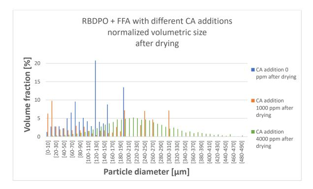
Figure 77 The normalized volumetric size distribution for the samples containing FFA with different CA additions. The samples are measured after drying.
