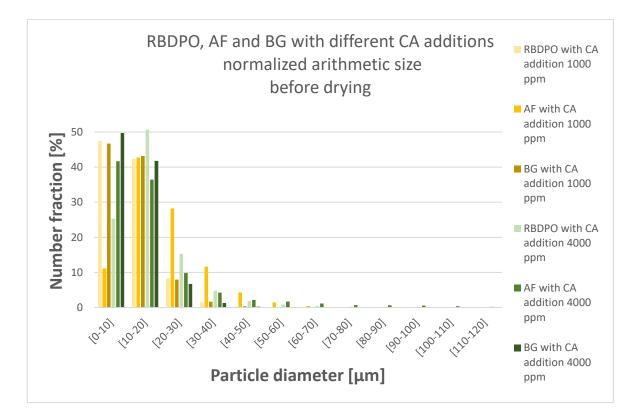
Figure 104 The normalized arithmetic size distribution for the samples of different feedstocks containing 1000 ppm or 4000 ppm of CA. The analysis has been performed before drying.
