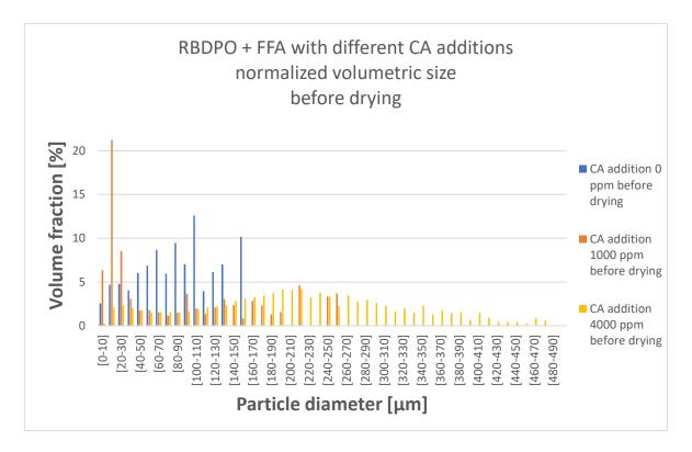
Figure 76 The normalized volumetric size distribution for the samples containing FFA with different CA additions. The samples are measured before drying.
