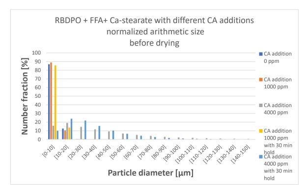
Figure 92 Normalized arithmetic size distribution for Ca-stearate experiments with different CA addition. The measurement was done before drying.
