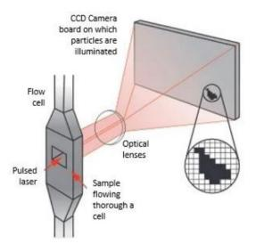
Figure 13 General principle of a dynamic image analysis (AZO Materials, 2019)
