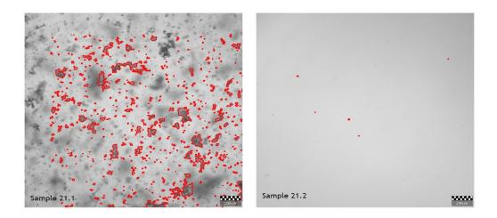
Figure 58 Exp 21, on the left there is the sample after acid treatment and on the right after filtration. Feedstock in the experiment is RBDPO and CA addition is 4000 ppm. The sample was left to rest in the heating closet 30 minutes before filtration.
