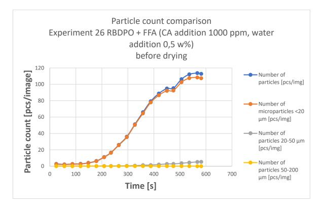
Figure 71 Particle count trend for the experiment 26, where FFA has been added to the solution.
