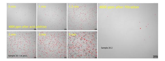
Figure 57 Exp 20, on the left there is the sample after acid treatment (6 pics) and on the right after filtration. Feedstock in the experiment is RBDPO and CA addition is 4000 ppm.
