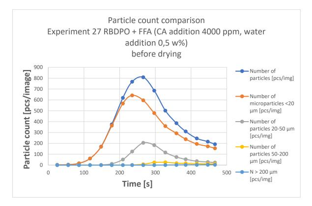
Figure 74 Particle count trend for the experiment 27, where the feedstock is RBDPO + FFA with CA addition of 4000 ppm.
