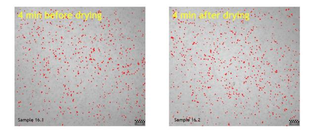
Figure 48 Exp 16, on the left there is the sample after acid treatment and on the right after drying. Feedstock in the experiment is RBDPO and the high shear mixer condition used in this experiment was 8000 rpm for 4 minutes.
