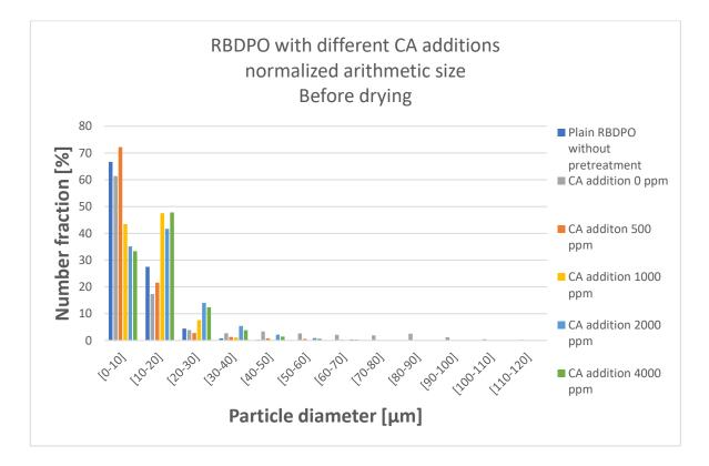
Figure 27 RBDPO with different CA additions, normalized arithmetic size data obtained from Pixact measurement. Data from the samples before the drying procedure.
