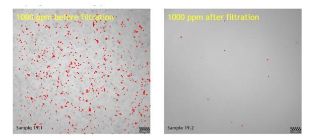
Figure 56 Exp 19, on the left there is the sample after acid treatment and on the right after filtration. Feedstock in the experiment is RBDPO and CA addition is 1000 ppm.
