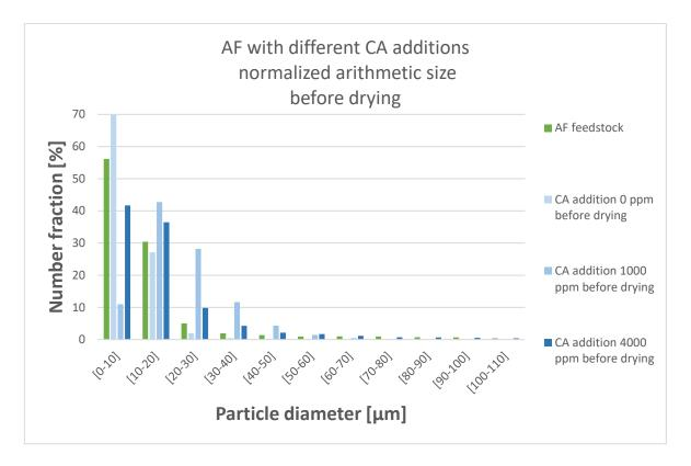
Figure 97 The normalized arithmetic size distribution for AF samples with different CA additions. The samples are measured before drying.
