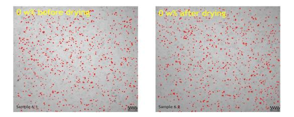
Figure 31 Exp 6, on the left there is the sample after acid treatment and on the right after drying. Feedstock in the experiment is RBDPO and the water addition 0 w%.
