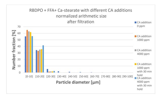
Figure 93 Normalized arithmetic size distribution for Ca-stearate experiments with different CA addition. The measurement was done after filtration.
