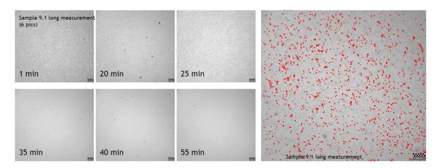
Figure 38 Exp 10 with prolonged Pixact measurement. On the left there is the sample after acid treatment (6 small pictures) and on the right after drying. Feedstock in the experiment is RBDPO and the water addition 2.0 w%. After 35 minutes Pixact measurement can recognize some small particles from the solution.
