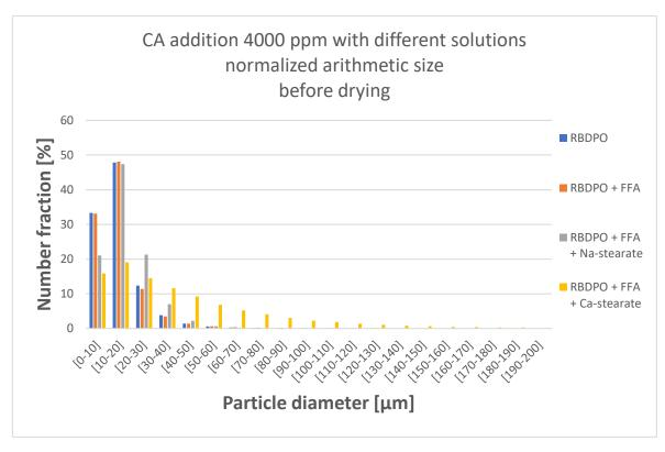
Figure 91 CA addition of 4000 ppm with different feedstocks, before drying procedure.
