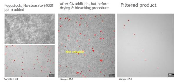
Figure 85 exp 34. Sodium stearate addition of 0,010 mol, CA addition 4000 ppm. Feedstock on the left side, product after acid treatment in the middle, filtered product on the right.
