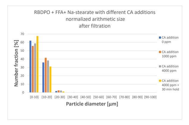
Figure 87 Normalized arithmetic size distribution with the samples containing RBDPO, FFA and Na-stearate. Samples have different CA additions, and they are measured after filtration.
