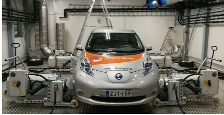
Fig. 1: Cold environment vehicle testing laboratory with the test subject car attached to a four-wheel dynamometer
