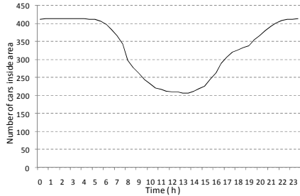
Fig. 3. Number of cars in the case area. The numbers are based on actual traffic flow measurement in the case area.
