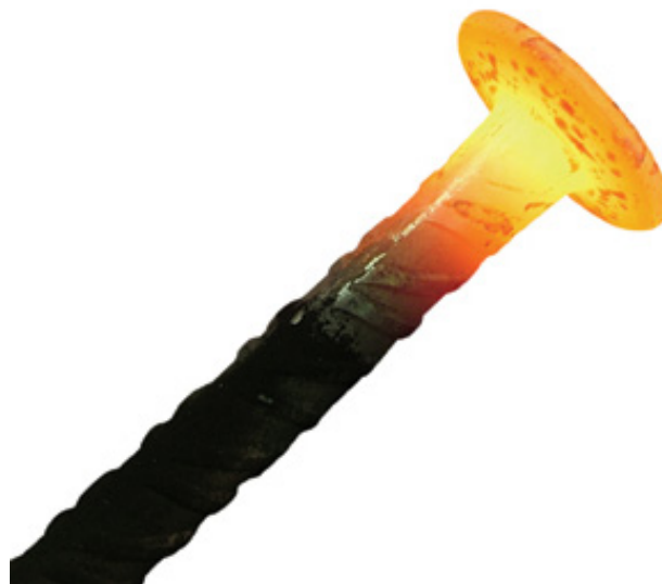
Figure 1: Hot upset forged headed rebar (LinkStudPSR 2023).
