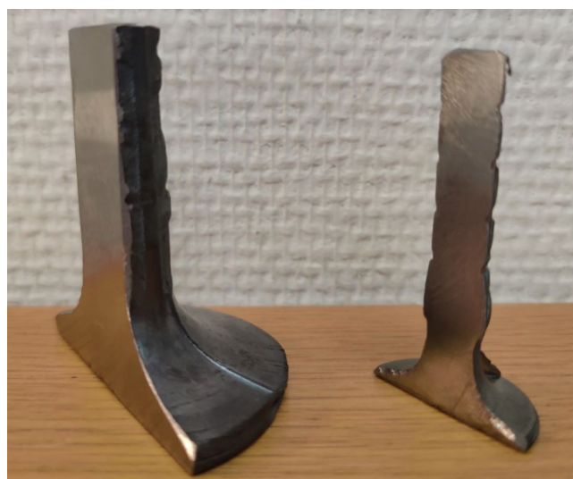
Figure 42: Milled testpieces for metallography and hardness measurements. 20mm rebar on the left and 10mm rebar on the right.
