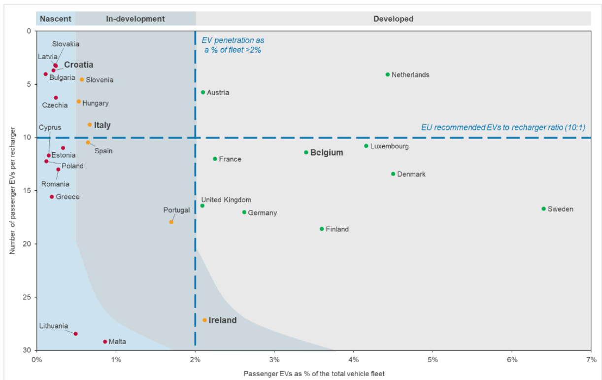
Figure 3. EU27 countries and the United Kingdom categorized by EVs per charging point and the EV share of total vehicle fleet. Data from year 2022. (adapted from European Commission 2023.) The term recharger in this context refers to a single charging point.
