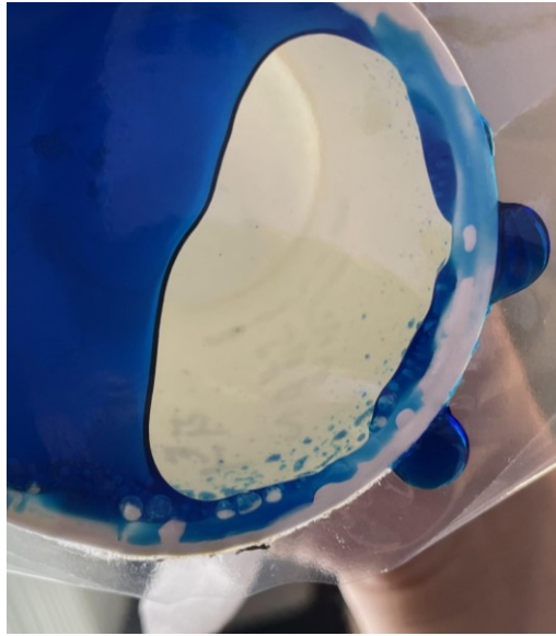
Figure 16. Bottom view of a flipped cup with dye water spreading
