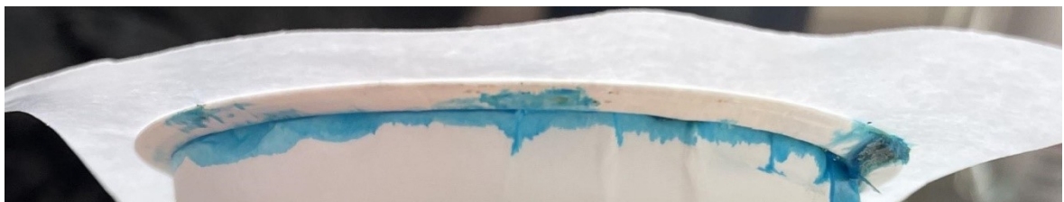
Figure 29. Liquid absorbed by cup wall
