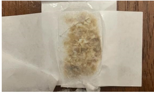
Figure 23. Paper+PE burned due to thickness increase
