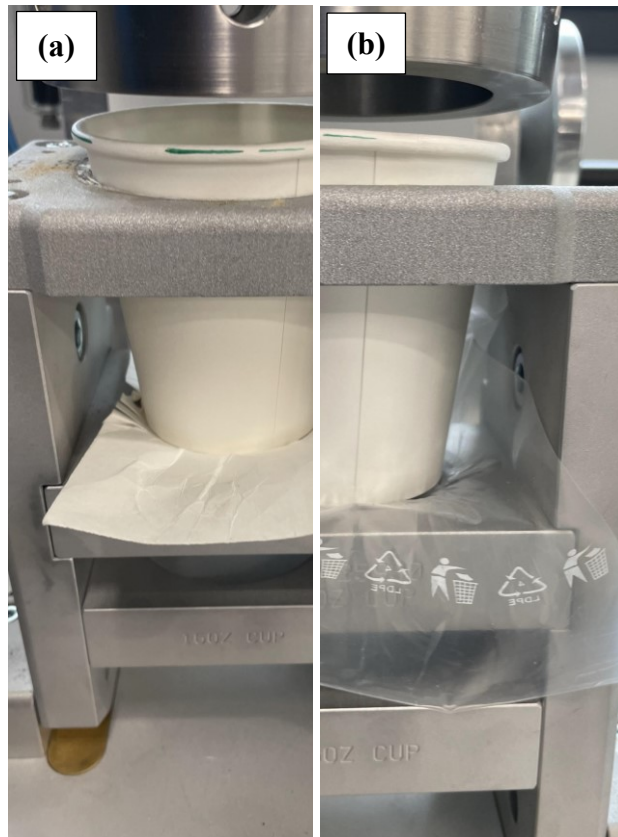
Figure 15. Cup removal. (a) thick material used. (b) thin material used.
