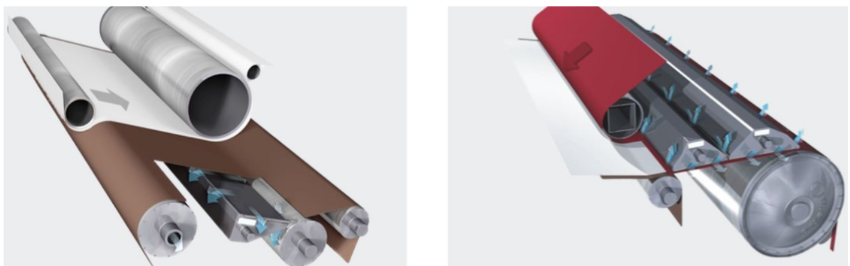
Figure 4. Press Nip and Press Run Web Stabilizers (Valmet Technologies 2020.)
