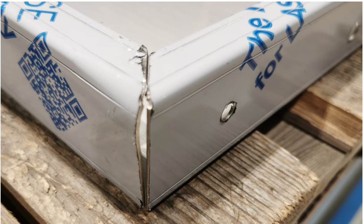
Figure 14. Welding gap number two
