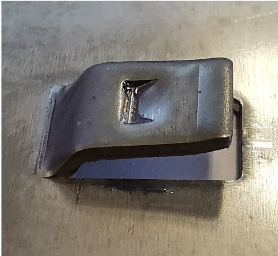
Figure 30. Sheet moulding made with available tool
