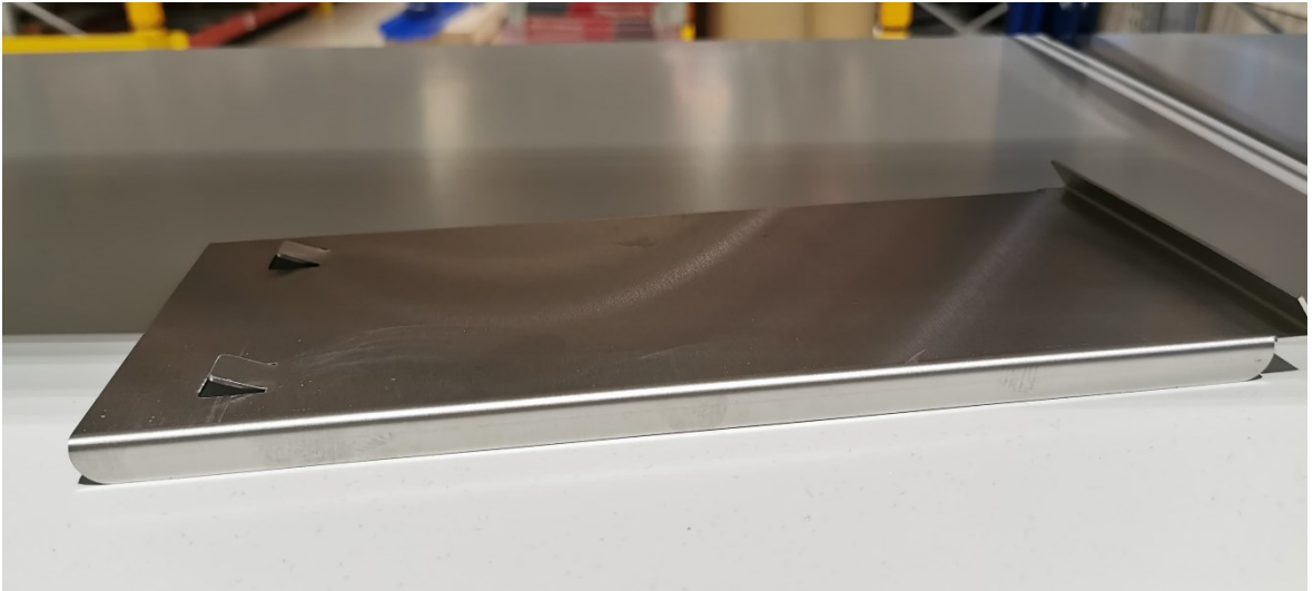
Figure 31. Blind filter with opened claws
