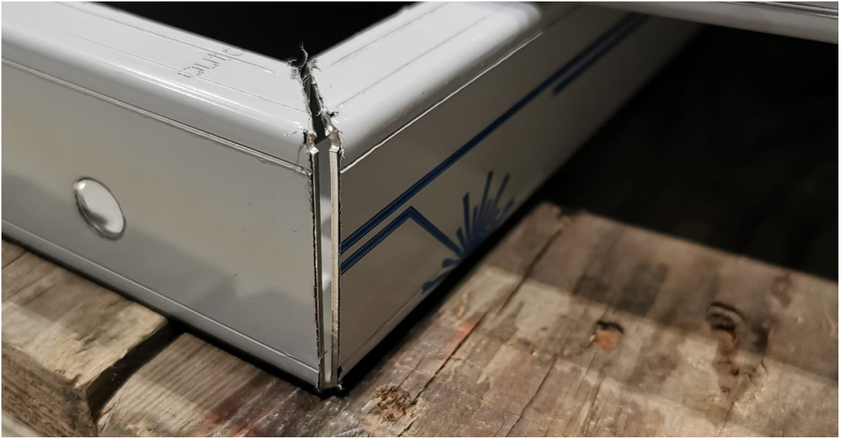
Figure 13. Welding gap number one
