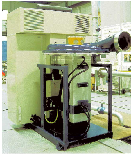
Figure 28: Test compressor used to investigate unsteady phenomena.
