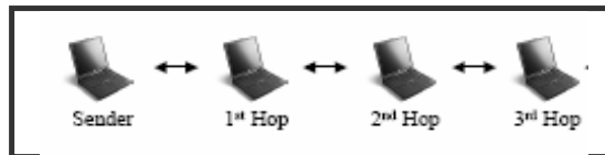
Figure 14: Linear Test Bed configuration for multi-hop multicast experiment
