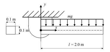
Figure 5. A free falling flexible pendulum for dynamic verification in the initial position.
