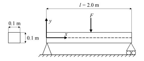
Figure 2. A simply supported beam for linear deformations.
