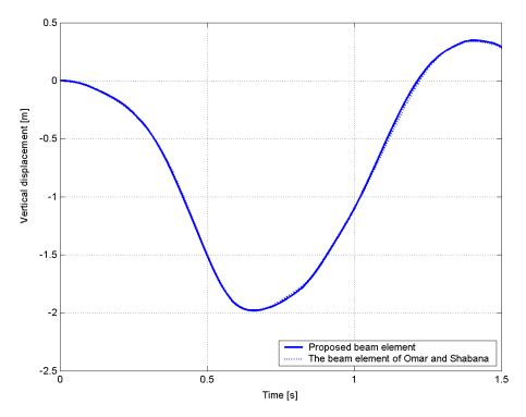
Figure 10. A comparison of the vertical displacement between the proposed element and that presented by Omar and Shabana using 8 elements.
