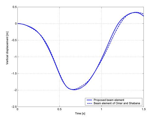
Figure 9. A comparison of the vertical displacement between the proposed element and that presented by Omar and Shabana using 4 elements.
