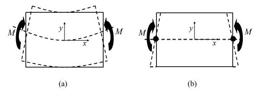
Figure 1. (a) The correct deformation mode of a rectangular block in pure bending.
