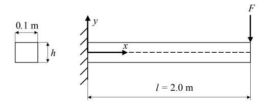
Figure 3. The cantilever beam model for nonlinear deformations.
