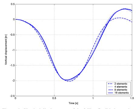
Figure 6. Vertical displacement of the falling flexible beam tip point using 2, 4, 8 and 16 elements.
