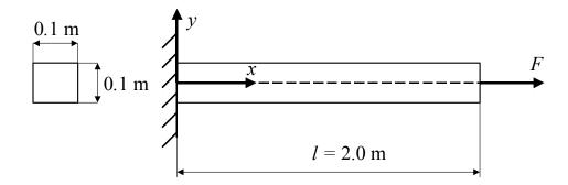
Figure 4. The cantilever beam model for linear axial deformations.
