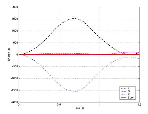
Figure 7. The energy components and energy balance of the falling flexible beam made up of 4 elements.
