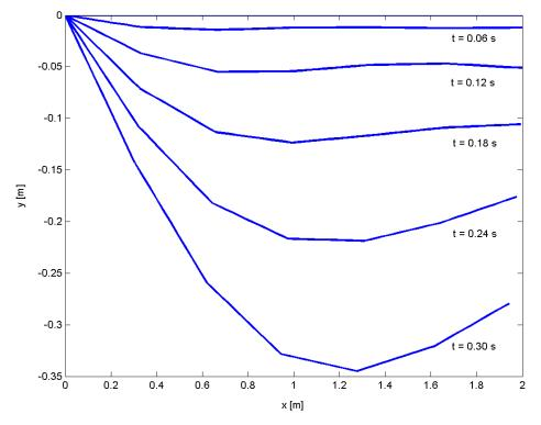
Figure 8. The falling flexible pendulum at different time steps under the effect of gravity using 6 elements.
