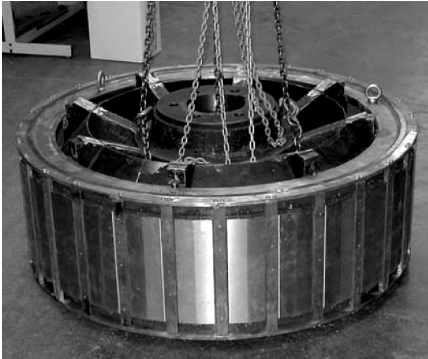
Fig. 2.10. Rotor of the 310 kW direct-on-line permanent magnet synchronous generator provided with damper windings around the permanent magnets (Va Tech Hydro 2007).
