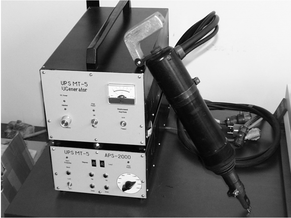
Figure 3.2 27 kHz ultrasonic impact treatment equipment
