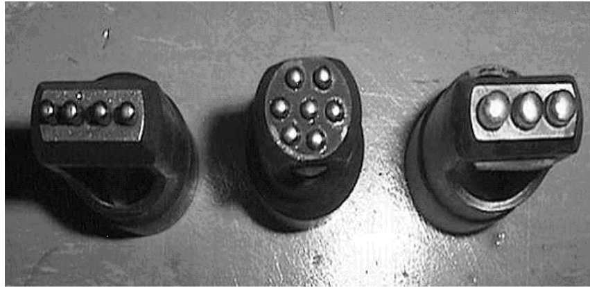
Figure 3.4 Several examples of needle sizes and configurations for the UIT device
