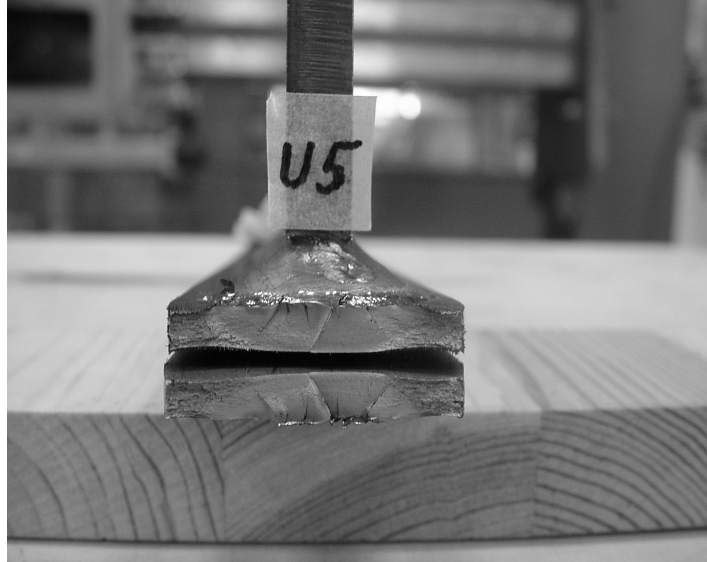
Figure 6.10 Cross section and crack shape of specimen (UIT-5) broken from UI –treated groove.
