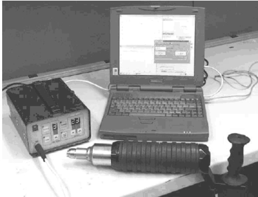
Figure 3.9 A UP device manufactured by Integrity Testing Laboratory (Kudryavtsev and Kleiman 2005).
