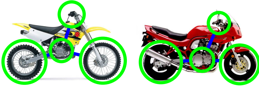
Figure 2.1: An example of object class detection with “parts and structure” model. Same parts – tires, motor and handlebars – of two motorcycles are marked by green circles and their spatial relationships with blue lines.
