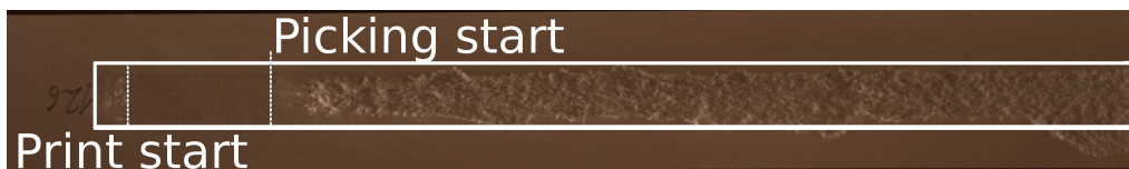
Figure 4.4: Different areas of a picking sample. Printed area is marked with a thick borderline. The start of the printed area contains some picking due to initial impact of the printing head on the paper.
