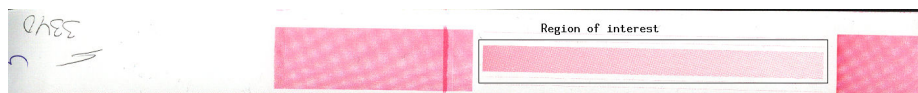
Figure 2.2: Sample Heliotest strip with the measurement area, i.e. the area where the missing dots are measured, (110mm \times 8mm) marked on the image.
