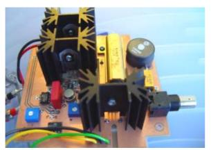
Fig. 11: Prototype converter for experimental tests built in our laboratory.
