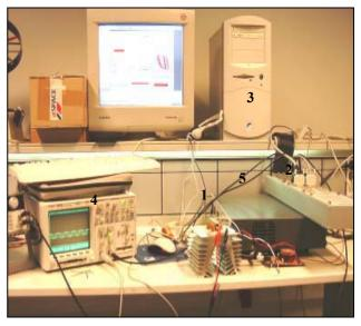
Fig.4. Test set-up consisting of the: Buck-Boost converter (1), connector panel (2), host pc with dSPACE<sup>TM</sup> DS1103 card (3), oscilloscope (4), and input voltage source (5).
