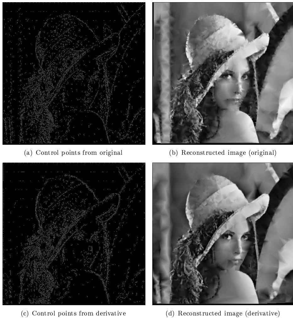
Figure 6.1: Example of DTOCS image compression. Image (b) is reconstructed from the 6944 control points shown in image (a), and image (d) from the 6847 control points shown in image (c). The original image contains 512 \times 512 pixels, so only about 2.6 % of the gray-values plus their relative locations are stored in the compressed images.
