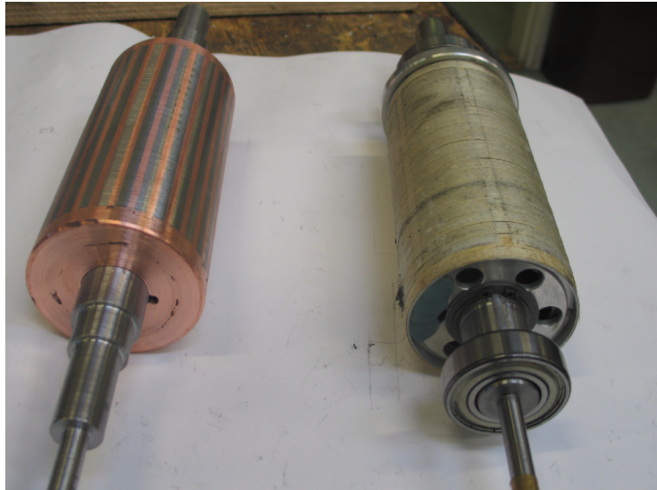
Figure 2.5. The rotors of the two motor types used in this study. On the left, there is the newly designed copper-cage rotor, and on the right the original PM rotor. The PM rotor is surrounded by a fibre-glass band to provide large enough mechanical strength.
