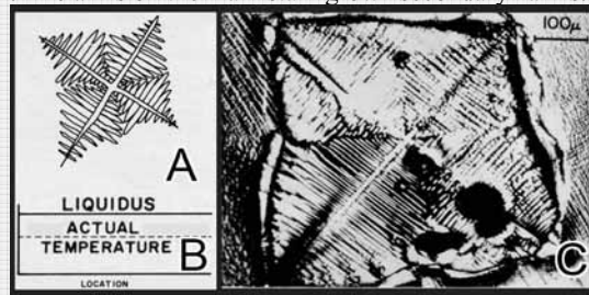
Fig. 2.24. A: Equi-axed dendritic mode of solidification. B: Temperature gradient G practically horizontal. [34] C: Photomicrographs of an equi-axed dendritic microstructure. Savage, Nippes, Miller 1976 [34] and Savage 1980[12]
