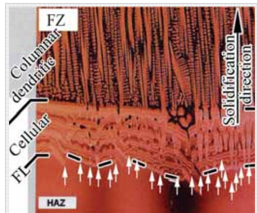
Fig. 5.11. Fusion line/weld interface FL, Cellular and columnar dendritic areas and cells (white arrows) as marked by the author on a micrograph of a Ni-superalloy spot weld. David, Babu, Vitek2001 [105]. No distinct planar zone is detected.
