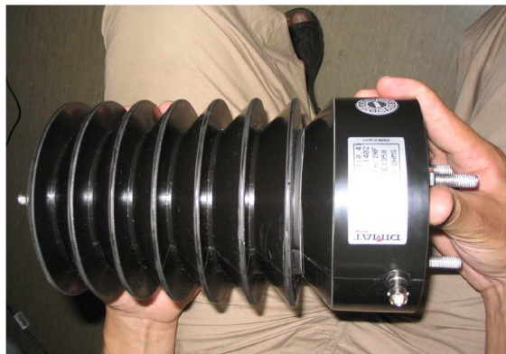
Fig. 3.11: Coupling capacitor for the MV distribution network.
