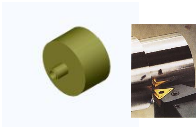
Stage 3. Turn in a lathe collar for the male connector and for the thread
