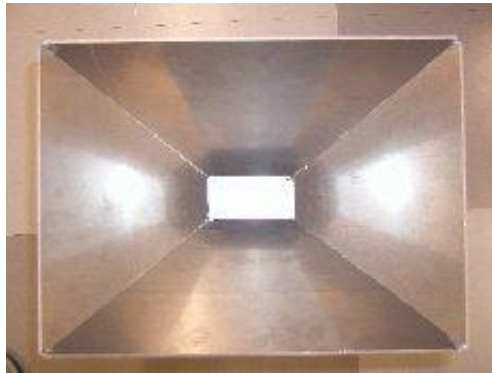
Fig 11.1 TIG-welded antenna body. The geometry of the open end of the conical horn antenna looks acceptable.
