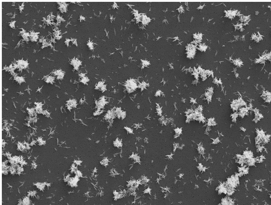
Figure 11. SEM image of clustered aragonite, 50 mg/l filtrated, ultrasound m03 10min, 1000x SE.
