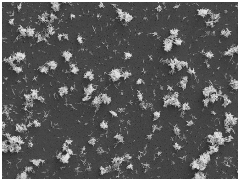
Figure 65. SEM image of clustered aragonite, 50 mg/l, m03 ultrasound, 1000x SE.
