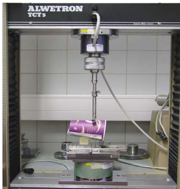
Figure 12. Grip stiffness test arrangement.
