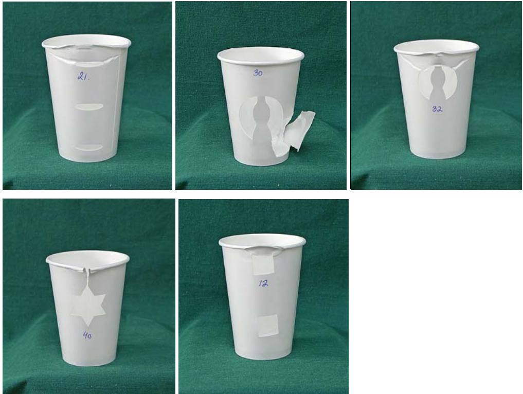
Figure 16. Some examples of unacceptable cups after cup machine.
