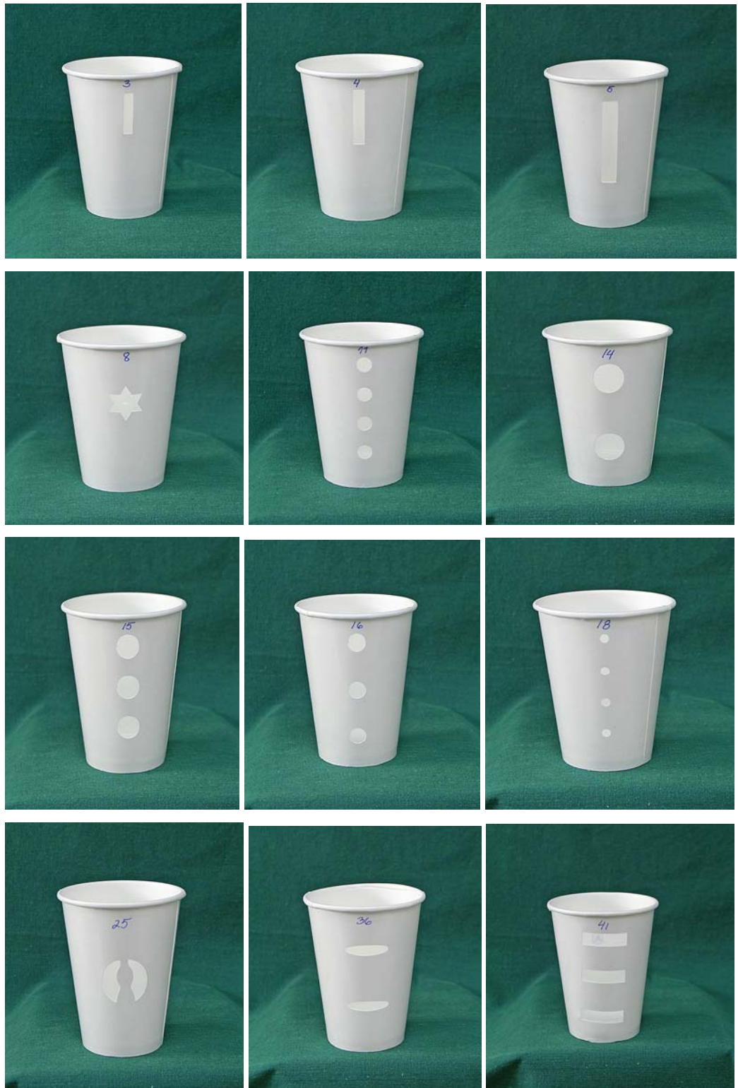
Figure 14. Acceptable cups after cup machine.
