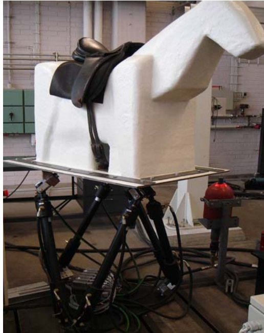
Figure 19. A horse simulator with Stewart- Gough mechanism developed in LUT
