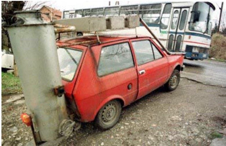
Picture 1. Yugo 45 runs on wood gas (Zastava Yugo Page)
