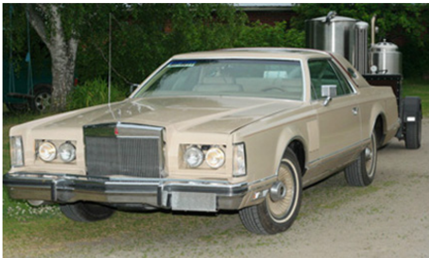
Picture 2. Lincoln Continental runs on wood gas (Renewable Energy for Housing and Transportation 2008)
