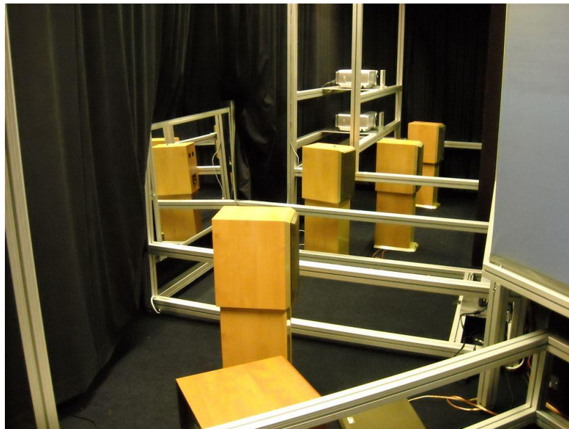
Fig.2.7 Speakers and subwoofers behind the rear projection screens
