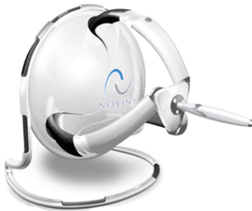
Fig.2.9 Parallel kinematics haptic device (Novint 2009)
