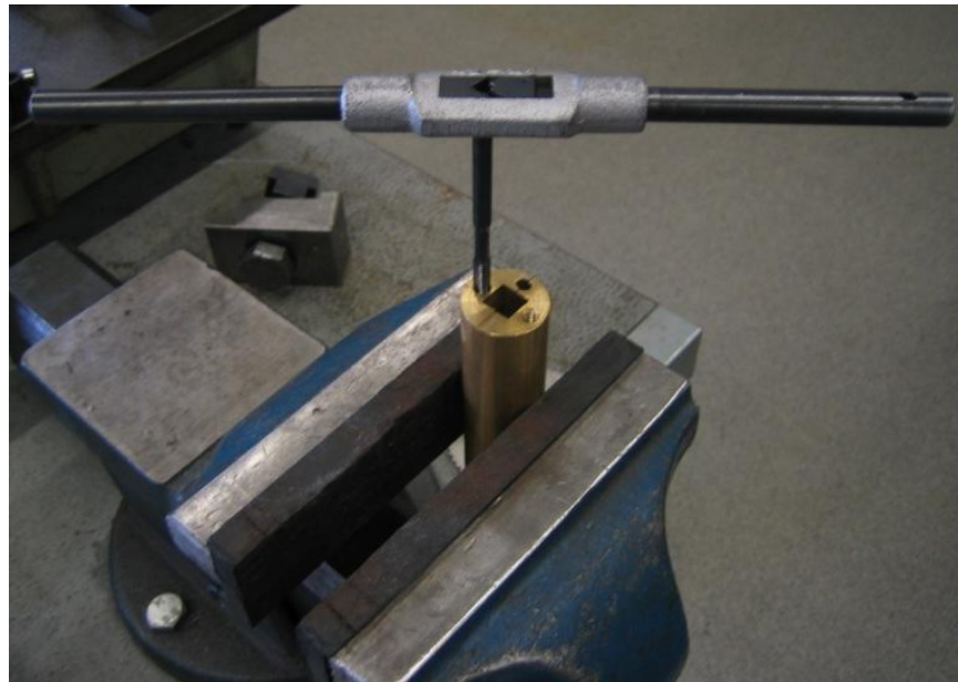
Figure 36. A hand-held thread carving tool.
