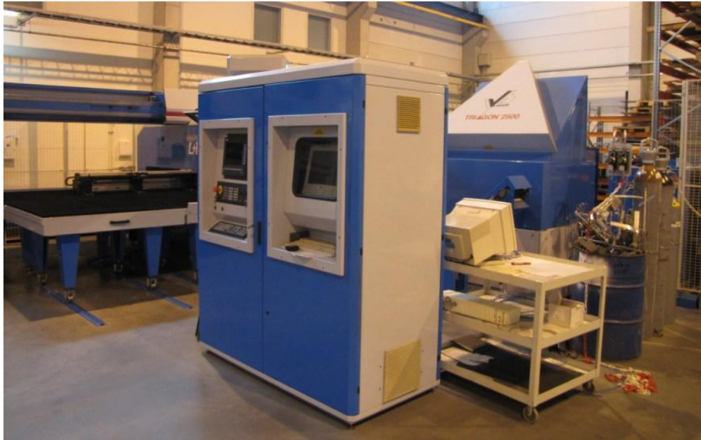
Figure 34. Finnpower sheet metal machining center. Triangular part is the laser resonator.
