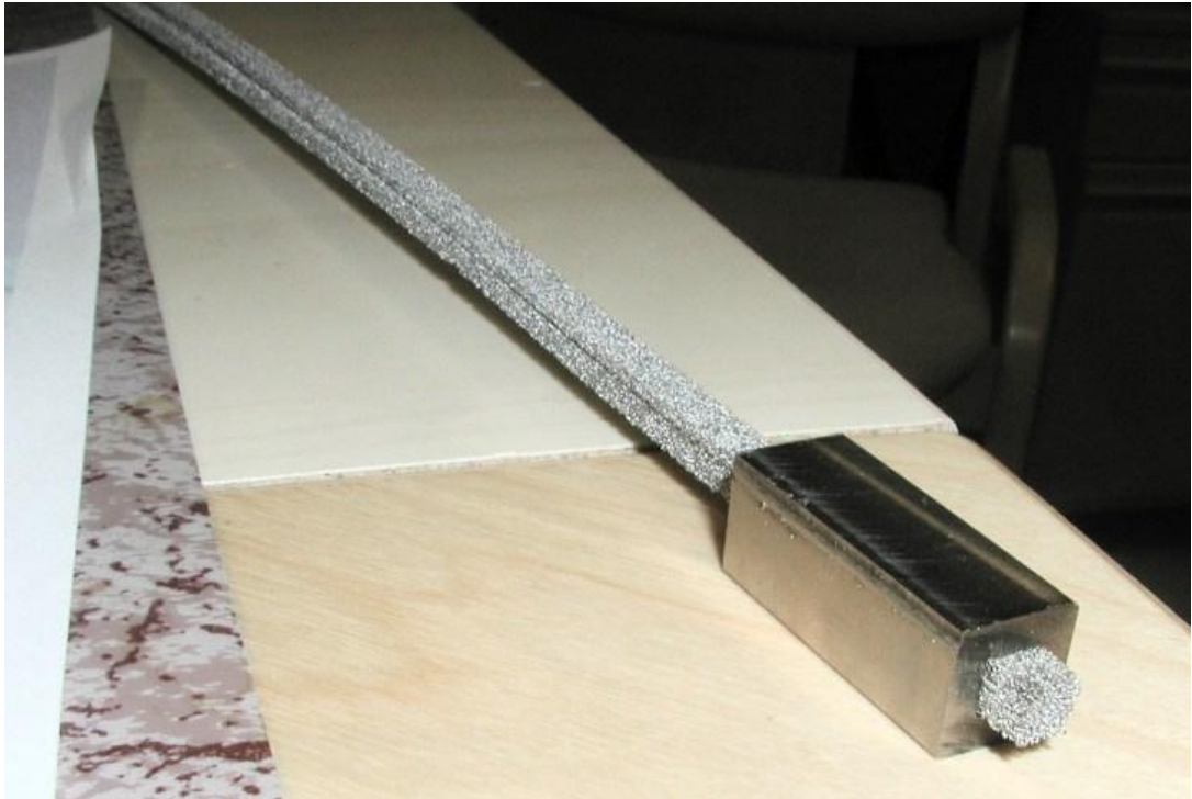
Figure 42. Metal foam inside the test chamber, cut with a 200W fiber laser.
