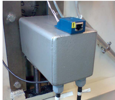
b) Slide ring at the end of grooved roll shaft. Figure courtesy of Miulus & Mattila/TUAS.
