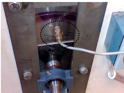
Figure 46: a) Trigger sensor. Figure courtesy of Miulus & Mattila/TUAS,
