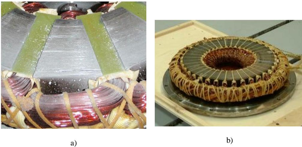
Fig. 1.1. a) End winding of a concentrated winding machine and b) an integral slot winding machine
