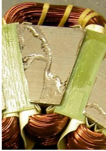
Fig. 2.13. End winding of a double-layer concentrated winding.
