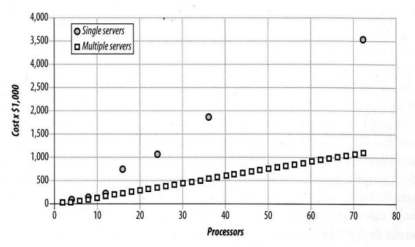
Figure 3. Costs of scaling with a small number of powerful servers vs. with a large number of small servers Henderson (2006, p. 205).
