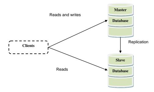
Figure 5. An example of master-slave replication sharing reads and master handling all the writes (Henderson, 2006, p. 233).
