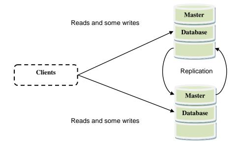
Figure 7. An example of master-master replication in active-active mode (Henderson, 2006, p. 237).
