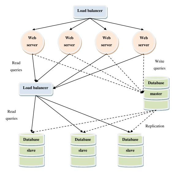
Figure 2. An example of application setup with hardware load balancing (Schwartz, et al., 2008, p. 437).
