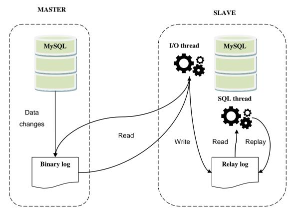
Figure 6. MySQL replication process (Schwartz, et al., 2008, p. 346).
