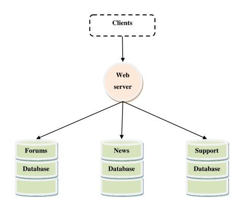
Figure 4. An example of functional partitioning for website with distinct sections (Schwartz, et al., 2008, p. 416).
