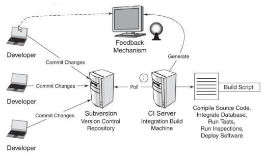
Figure 12: Components of CI system [38]
