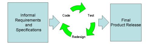
Figure 8: Code and Fix development model
