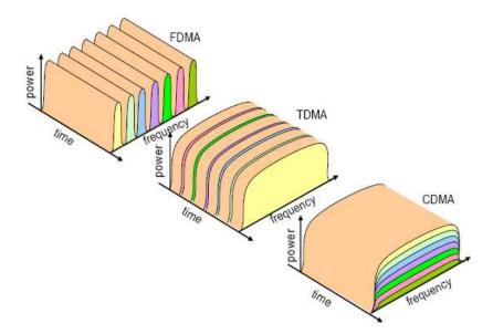
Figure 1: FDMA, TDMA and CDMA [7]
