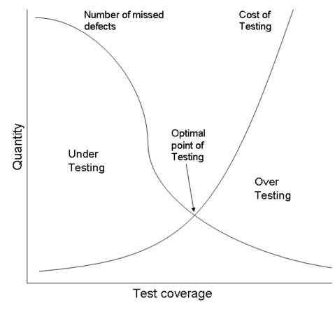
Figure 5: Optimal amount of testing [4]
