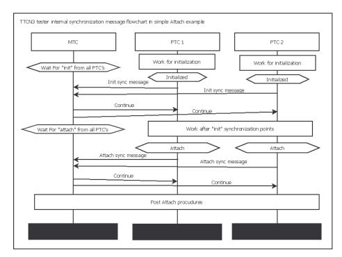
Figure 19: TTCN3 tester internal synchonization example
