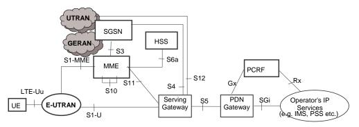
Figure 2: LTE network architecture [16]
