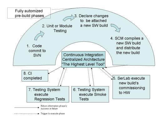
Figure 27: A centralized architecture for complete CI
