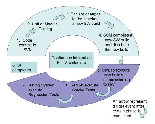
Figure 26: A Flat Architecture model in complete CI
