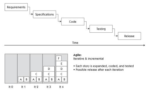
Figure 11: Agile versus Waterfall development model [22]
