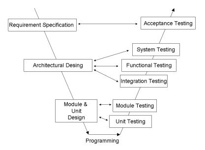
Figure 6: V-model of testing
