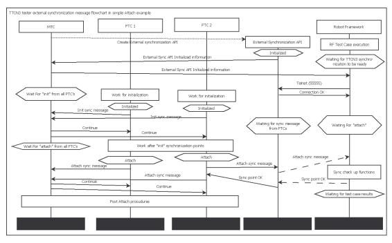
Figure 20: TTCN3 tester and RF external sychronization example
