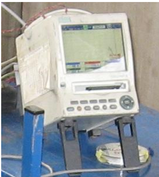
Figure 19. Yokogawa DR 130 data logger.
