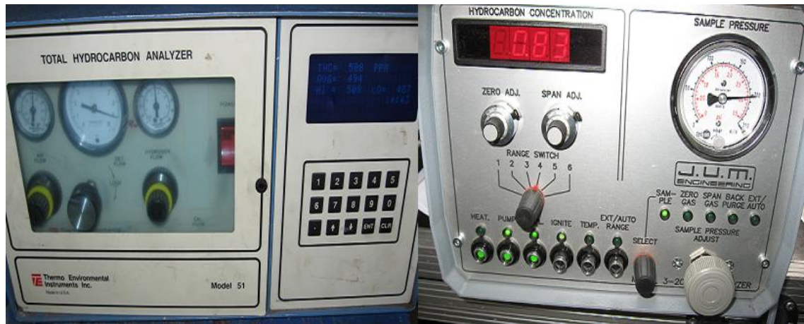
Figure 18. On the left is shown the T.E.I. FID and on the right is shown the J.U.M FID.
