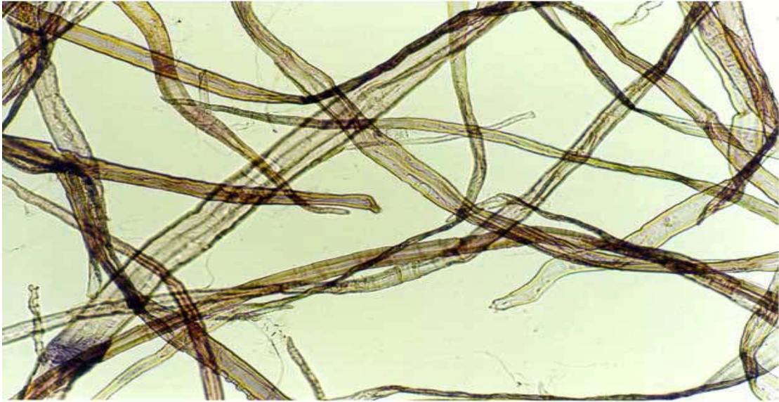
Figure 3. Softwood pulp (microscopic image enlarged 145x). (Knowpap, 2004)
