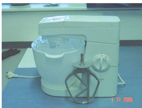
Figure 43. The commercial Kenwood kitchen mixer that was used for the mechanical treatment of the softwood kraft pulp.
