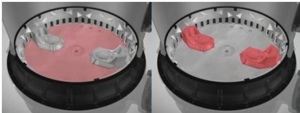
Figure 14. Grinding plate and lugs [10]
