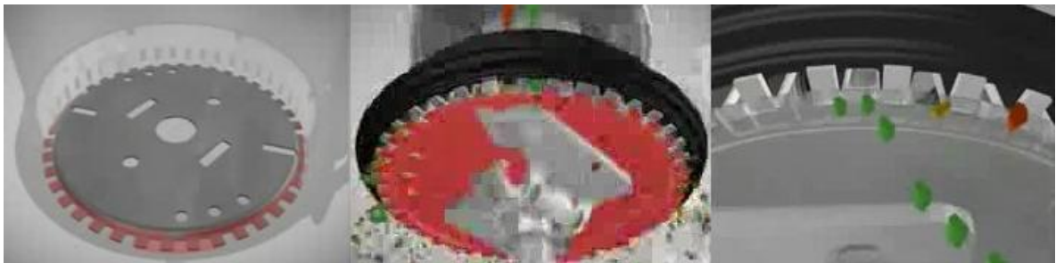
Figure 19.Undercutter disk cuts particles one more time [10]
