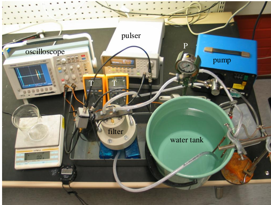
Figure 3.2: Photo of the ultrasound measurement setup. Arrangement of the instruments is the same as in Figure 3.1.
