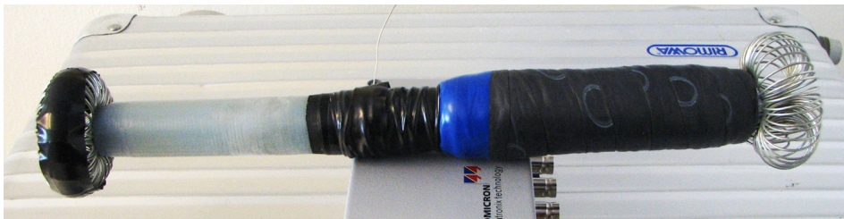
Fig. 3.8. Cable sample used in the partial discharge measurements. The white section is the insulation and the black cord is the ground conductor. The thick assembly on the right end contains cable termination. Conductive ring electrodes were added to reduce corona discharges. The thickness of insulation was 4.35 mm.
