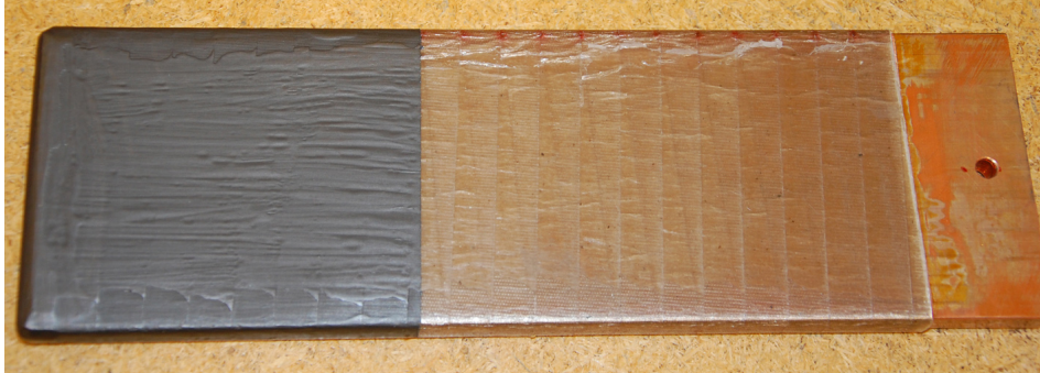
Fig. 3.7. Bar sample used in the partial discharge measurements. The black section is the ground electrode. The sample does not contain field grading.
