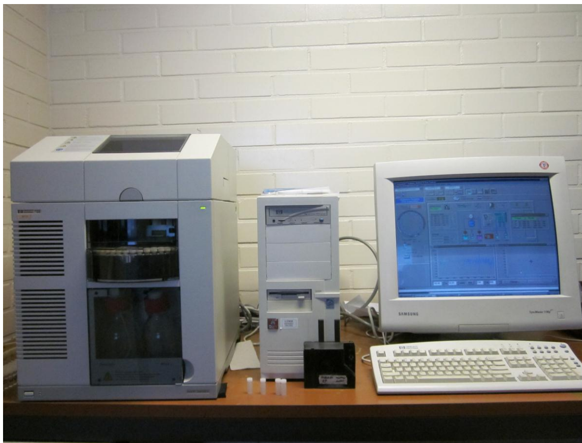
Figure 13. Instrumental set up of capillary electrophoresis system.
