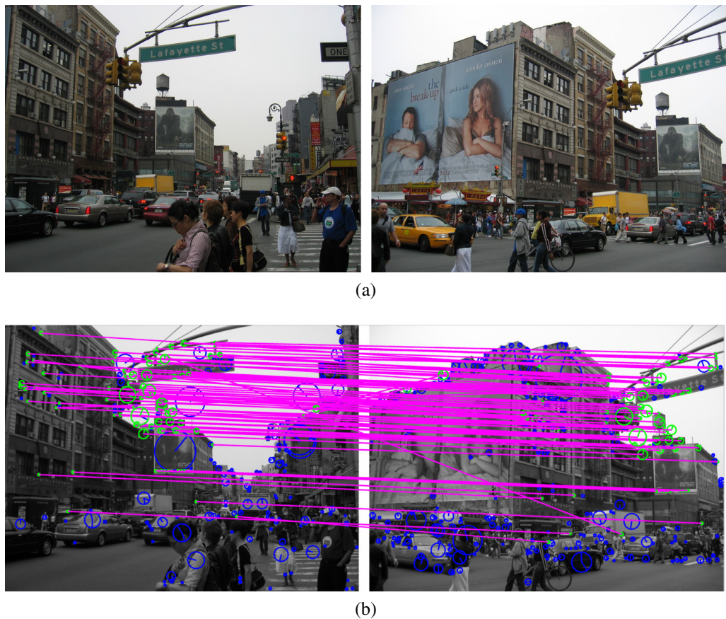
Figure 1. (a) An image pair showing a few buildings from two different viewpoints and (b) SIFT matches showing the corresponding features.
