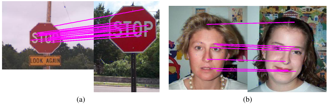
Figure 26. A matching example containing (a) LoG-vireo+SIFT-vireo descriptor matches on stop signs and (b) SURF+SURF descriptor matches on faces.
