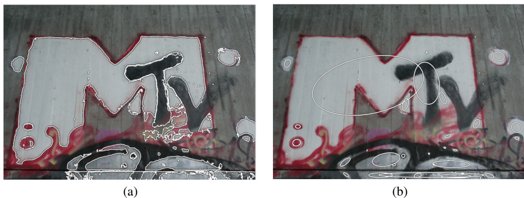
Figure 10. Local features detected with MSER. (a) The original MSER regions and (b) the fitted ellipses.
