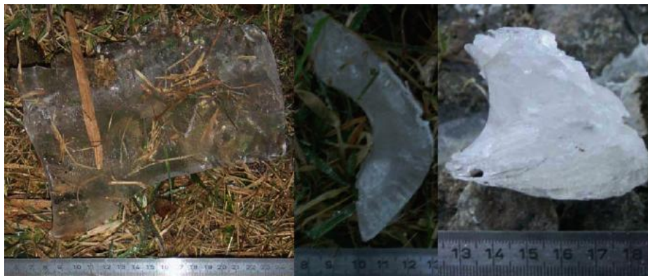
Figure 5.4.1 Examples of ice fragments found near wind turbines, or taken from blades (Homola M. C. 2005)
