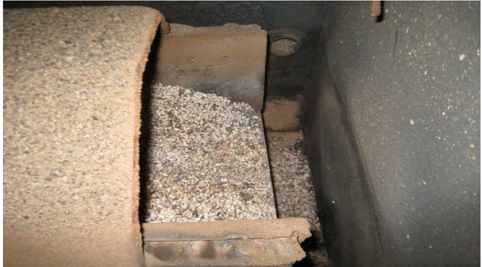
Picture 32. 100% MBM inside the furnace /67/.
