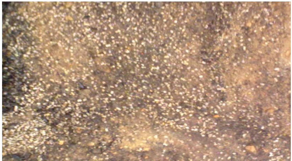
Picture 27. Ash of 90 % of peat and 10 % granulated MBM mixture /62/.
