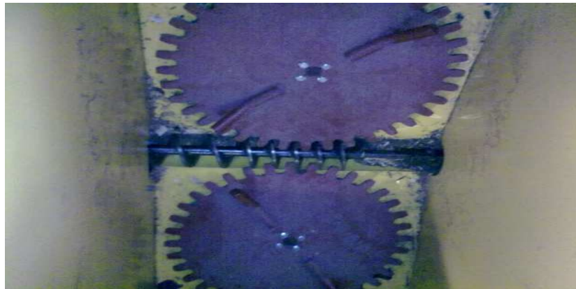
Picture 21. Fuel silo with screw conveyor /55/.
