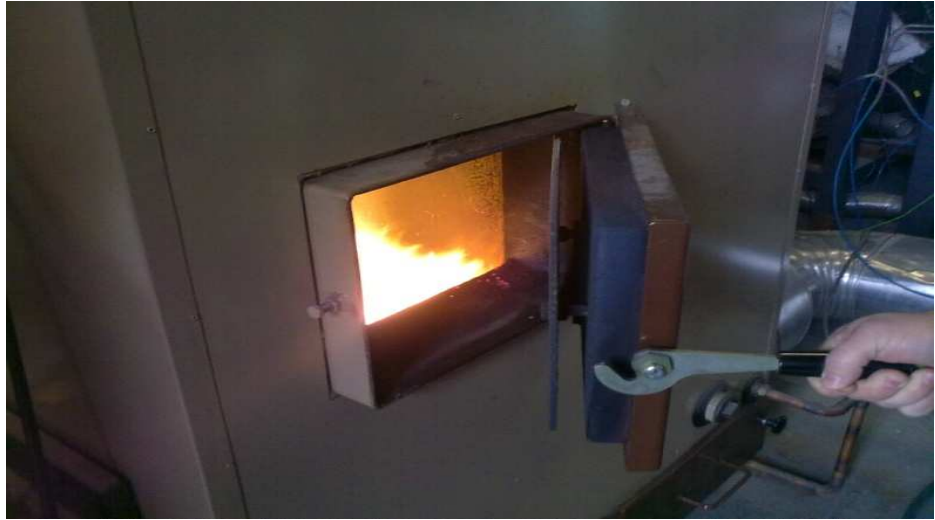
Picture 28. Burning process of 80 % peat and 20 % granulated MBM /63/.
