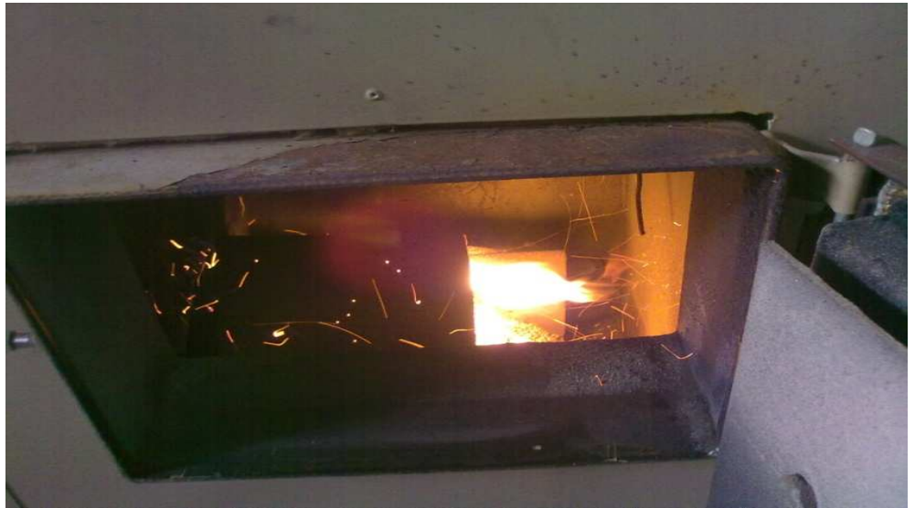
Picture 29. Pile of mixture inside the furnace /64/.
