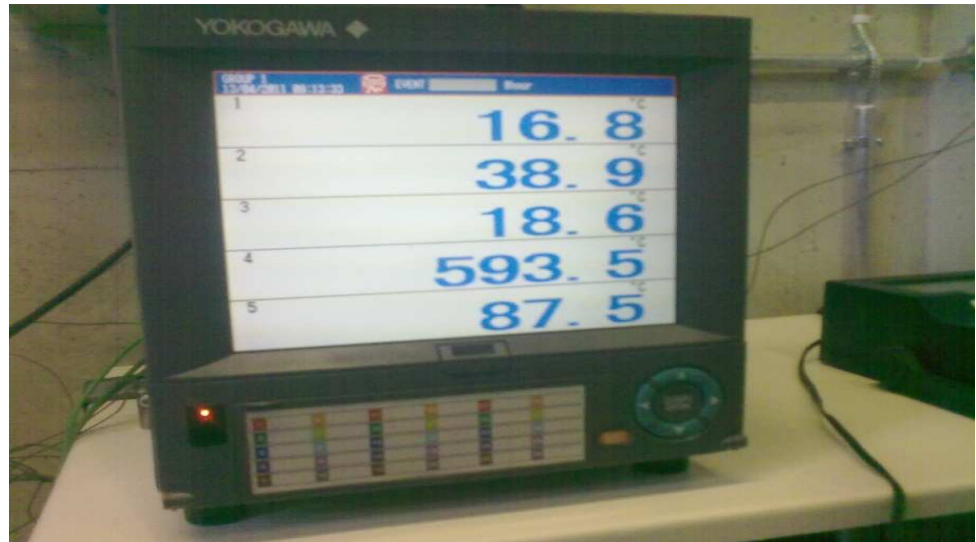
Picture 35. Temperature measurement device Yokogawa DX2030 /70/.
