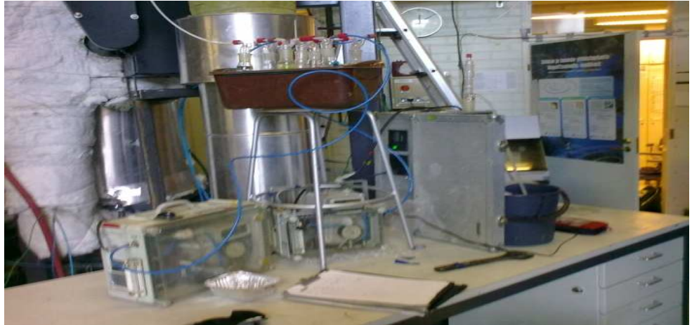
Picture 25. Heavy metal and PCDD/F measurement devices from flue gases /60/.
