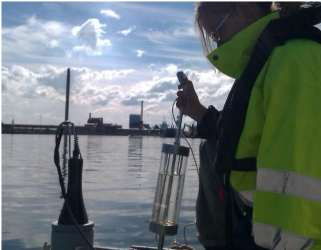
Figure 8.3. Ruttner water sampler with the turbidity monitoring equipment
