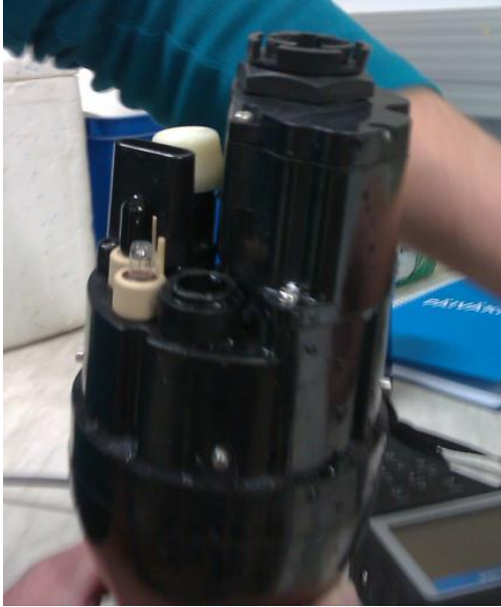
Figure 8.2. In-situ water quality measuring equipment for turbidity monitoring during dredging.
