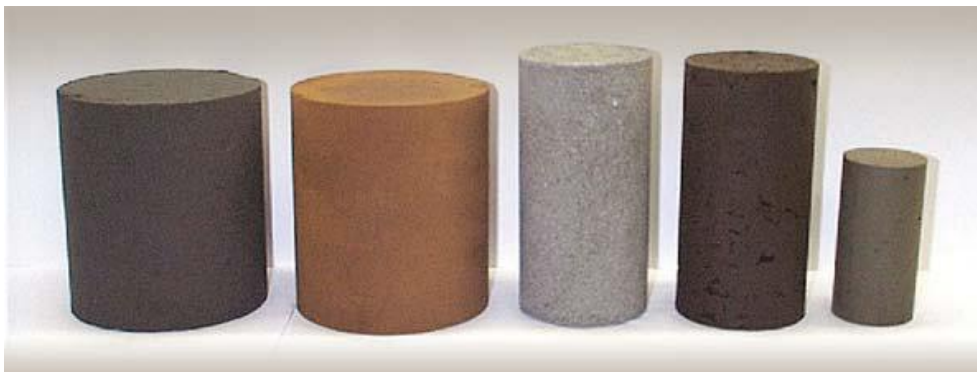
Figure 11.1. Specimens ready to unconfined compression test.
