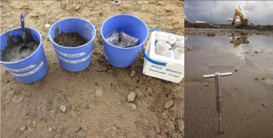
Figure 7.10. Original 0-mass, stabilized mass and samples taken from the mass in left, vane drill measurement in right.
