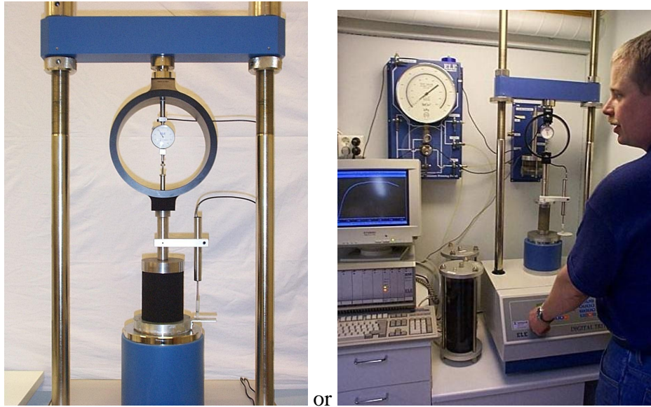
Figure 11.2. Unconfined compression test in progress. Ramboll Finland Oy.
