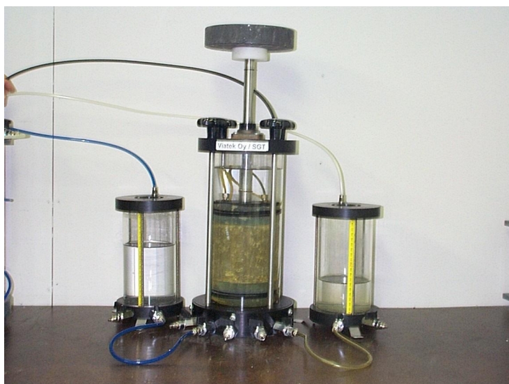
Figure 11.3. Permeability test in progress. Ramboll Finland Oy.
