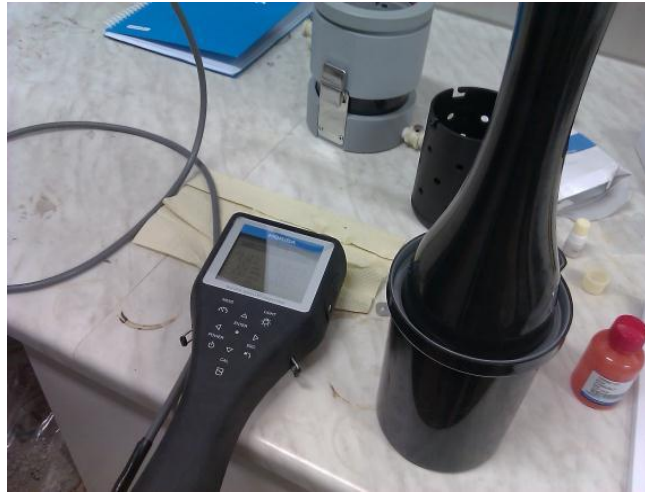
Figure 8.2. In-situ water quality measuring equipment for turbidity monitoring during dredging.
