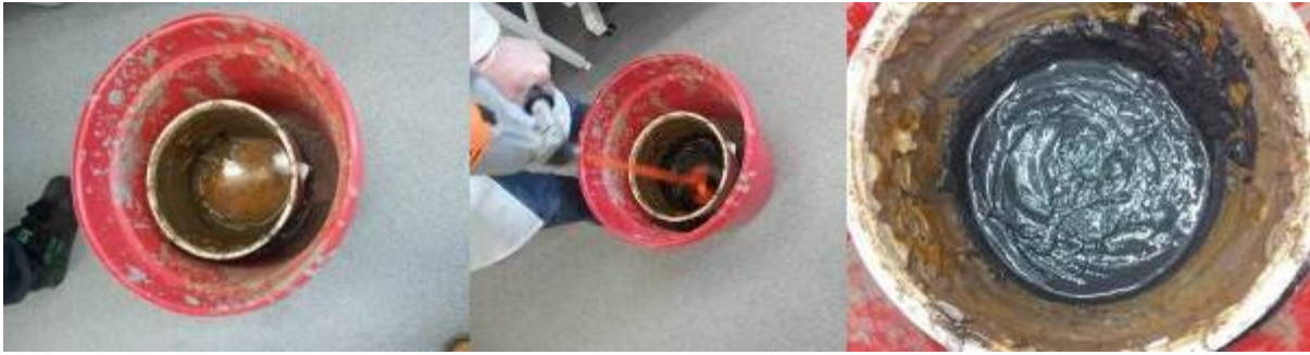
Figure 3.1 Homogenizing settled sediment material
