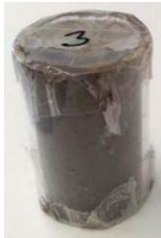
Figure 3.5 Acrylic test tube with stabilized sediment in it
