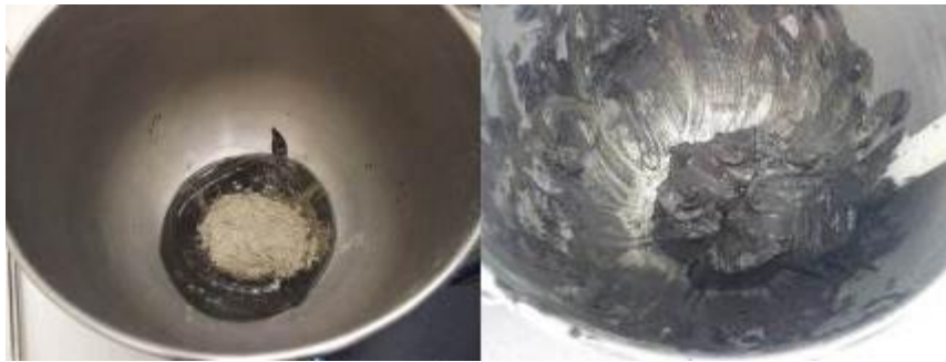
Figure 3.2 Sediment is mixed with dry binder materials
