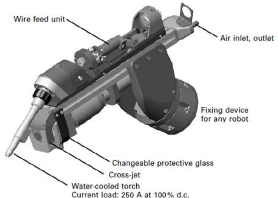
**Figure 2.3.7:** Schematic representation of a laser- MIG/MAG hybrid welding head [45].
