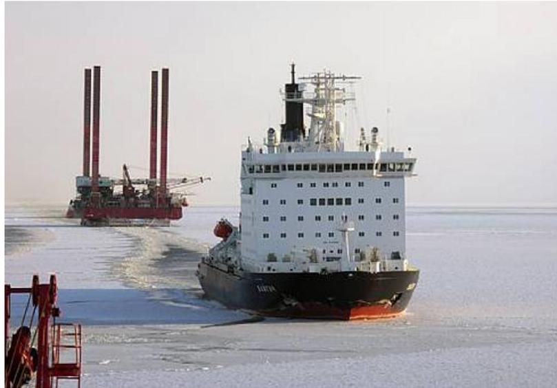
**Figure 4.1:** The nuclear-powered icebreaker 'Vaigach' towing an oil rig [65]
