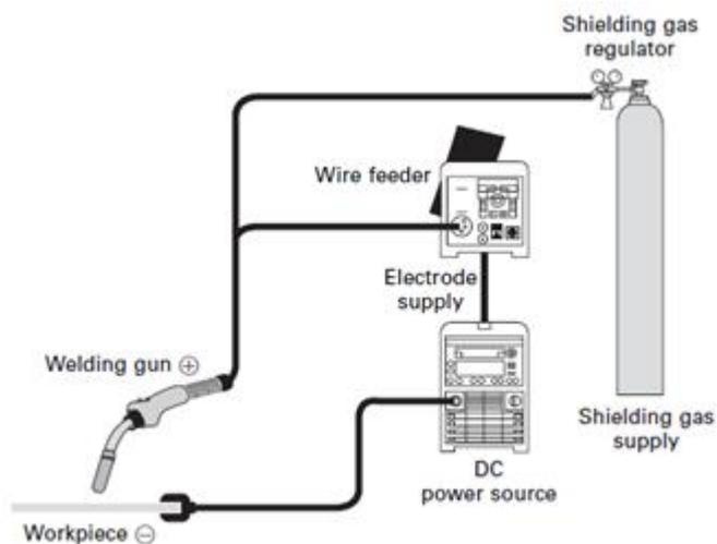
**Figure 2.3.9:** Schematic view of MIG/MAG welding system showing main components [45]
