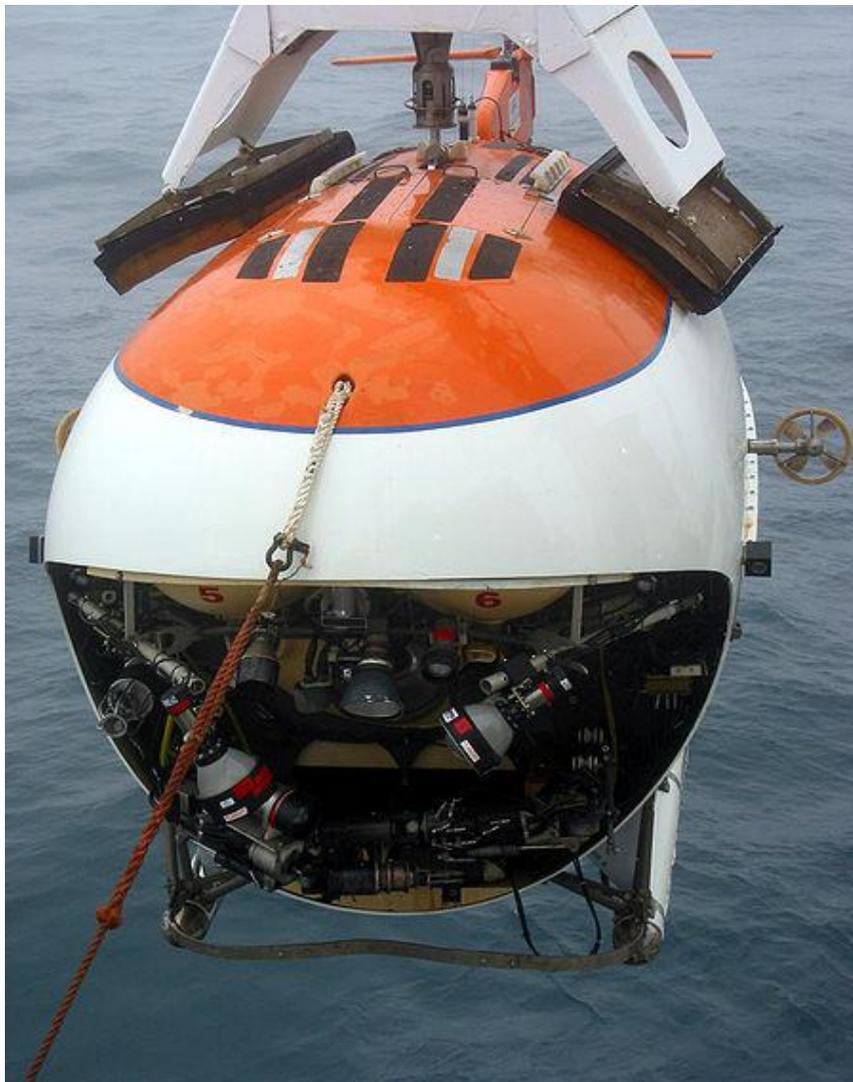
**Figure 1.3:** MIR submersible (deep-submergence vehicle)
