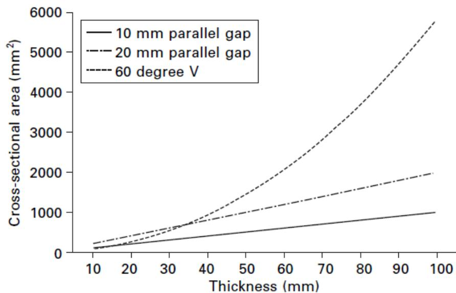
**Figure 2.3.2:** The principle of narrow-gap welding: The effects of joint preparation on weld cross-sectional area [24].
