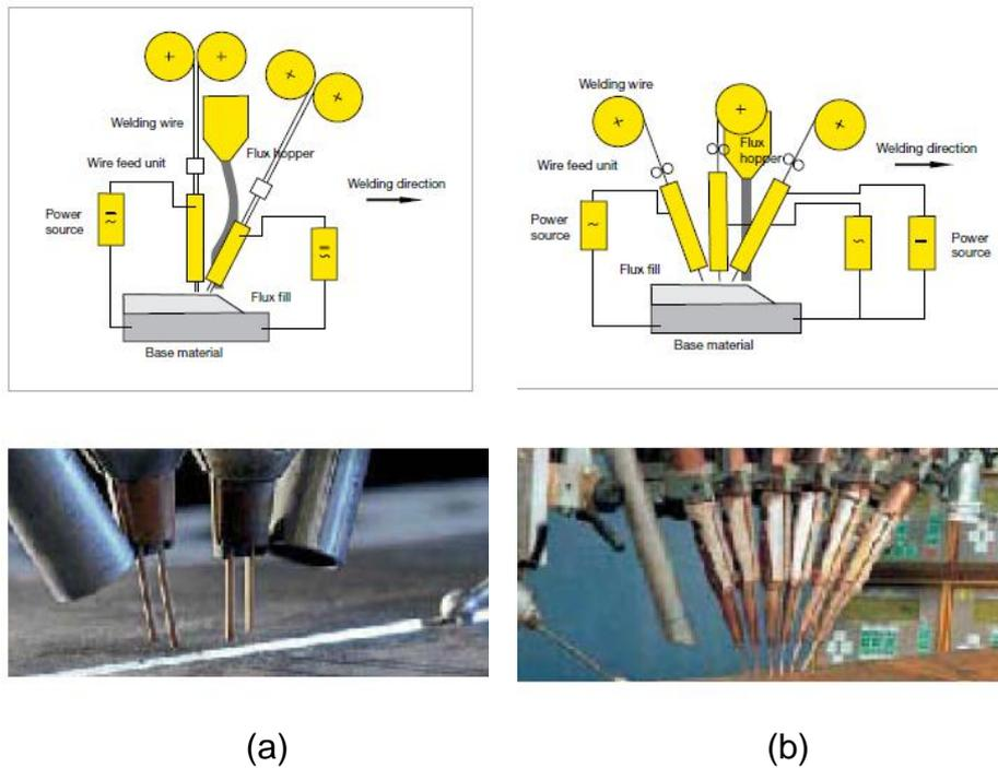
**Figure 2.3.18:** Twin Tandem wire variation (a) and Multiwire variation (b) [53]
