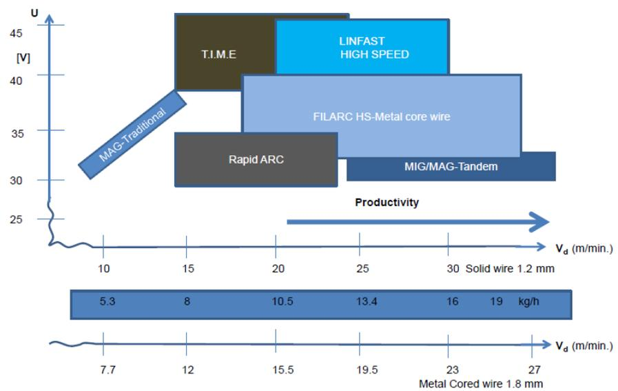
**Figure 2.3.12:** Comparison of different highly-productive MIG/MAG welding systems [48]
