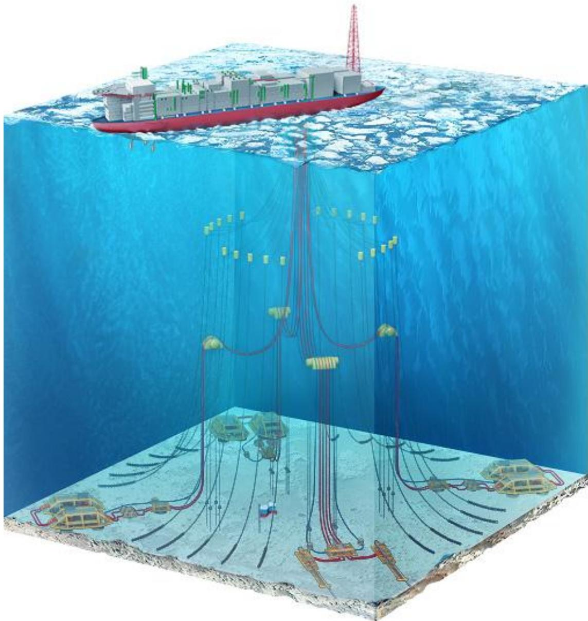
**Figure 4.3:** The offshore facilities for Shtokman project [63]
