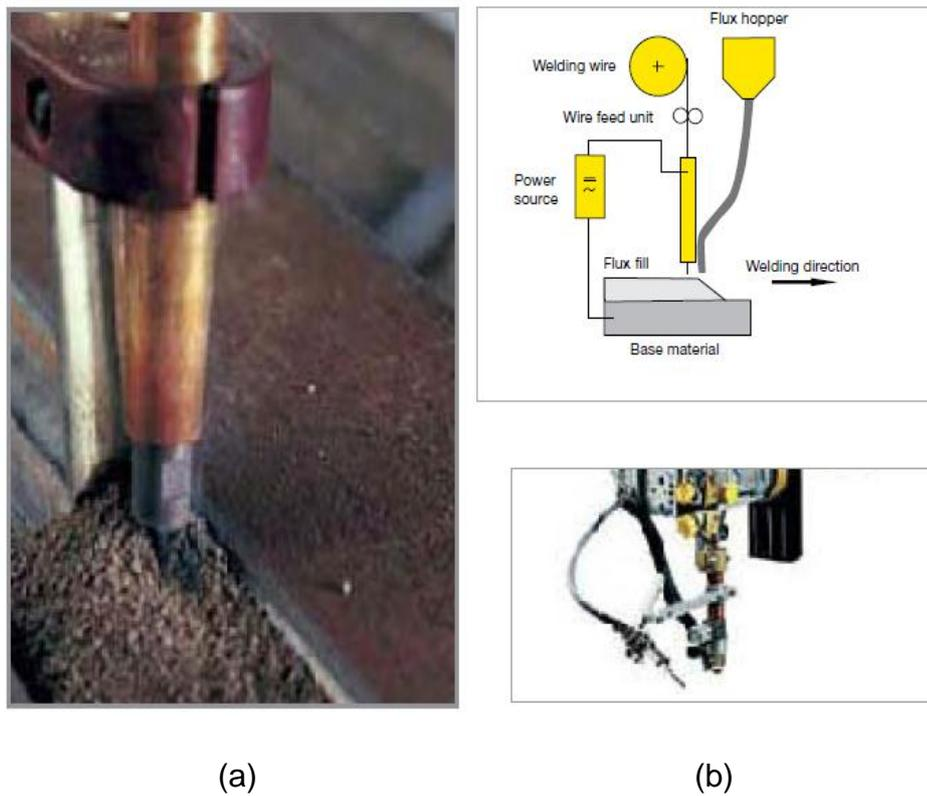
**Figure 2.3.16:** Core wire variation (a) and Single wire variation (b) [53]
