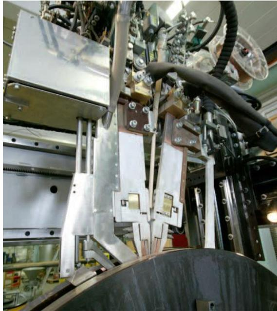
**Figure 2.3.3:** Narrow Gap Welding head [26]
