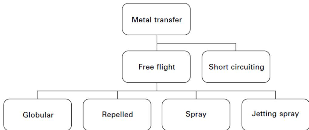
**Figure 2.3.11:** Classification of metal transfer in MIG/MAG [24]
