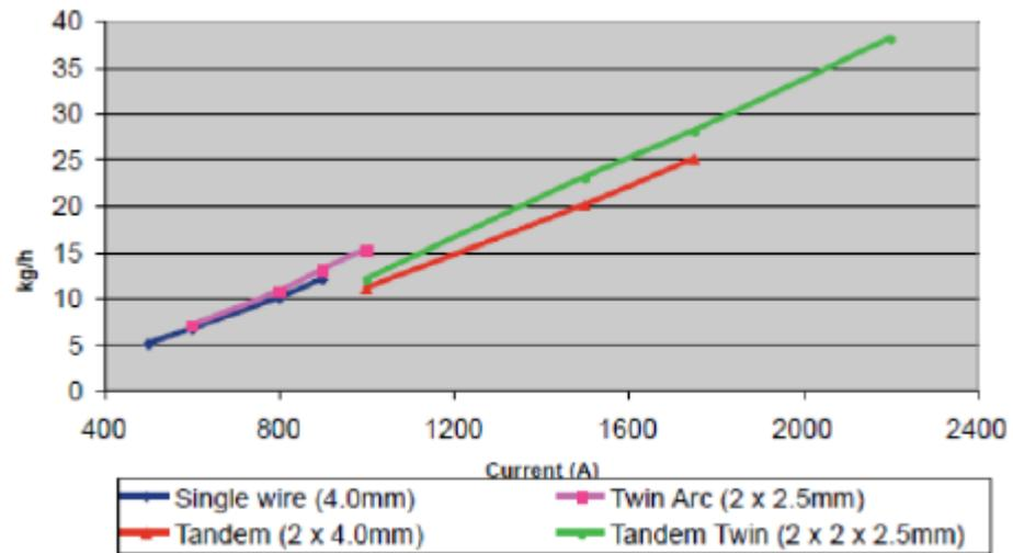
**Figure 2.3.19:** SAW process variations and their deposition rates [53]
