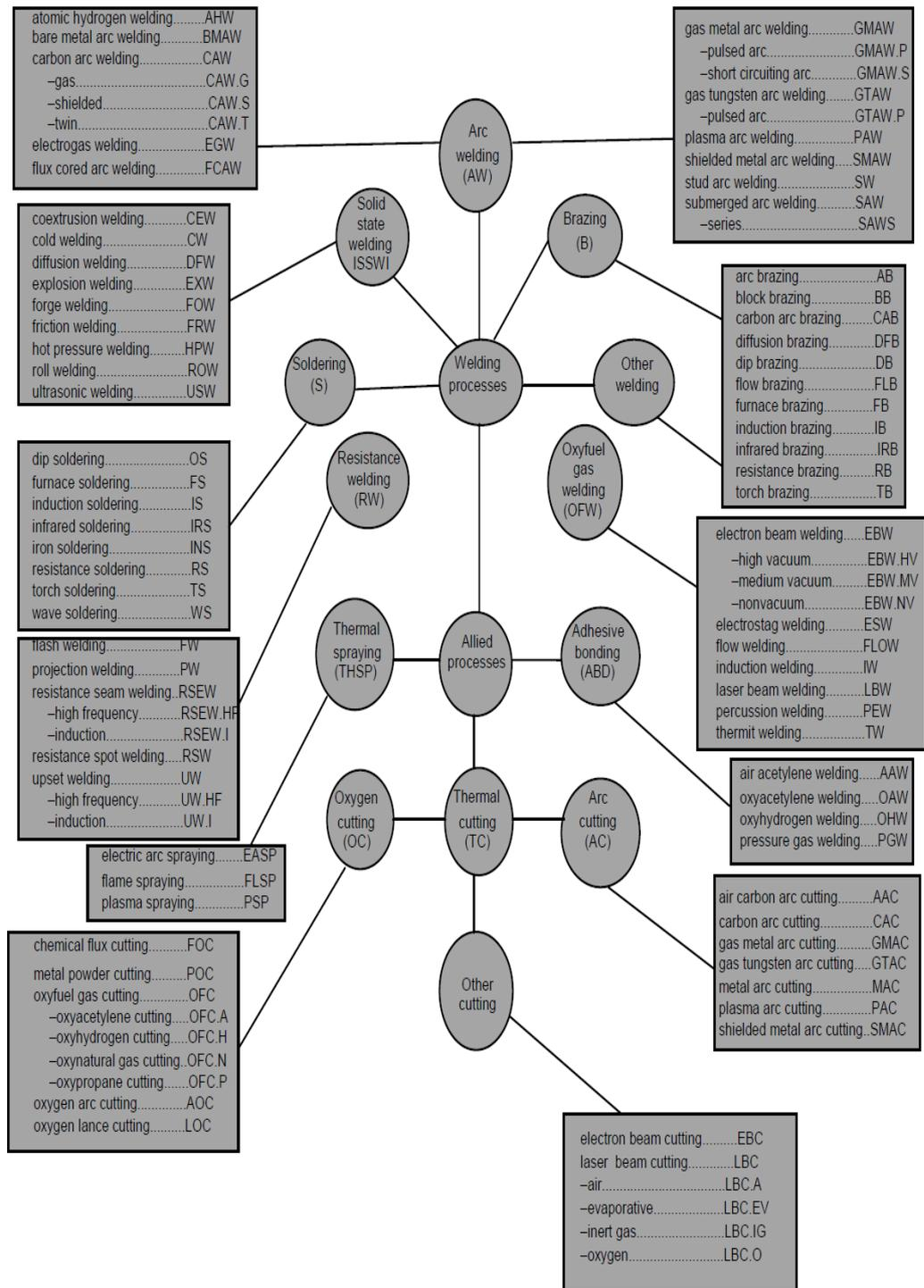
**Figure 1.1.1: Master Chart of Welding and Allied Processes**
