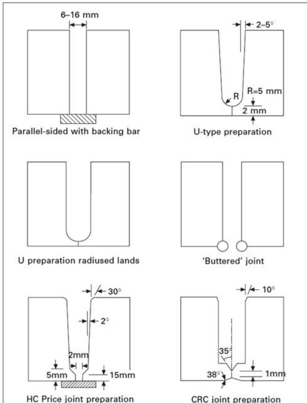
**Figure 2.3.1:** Typical narrow-joint Preparation. [25]
