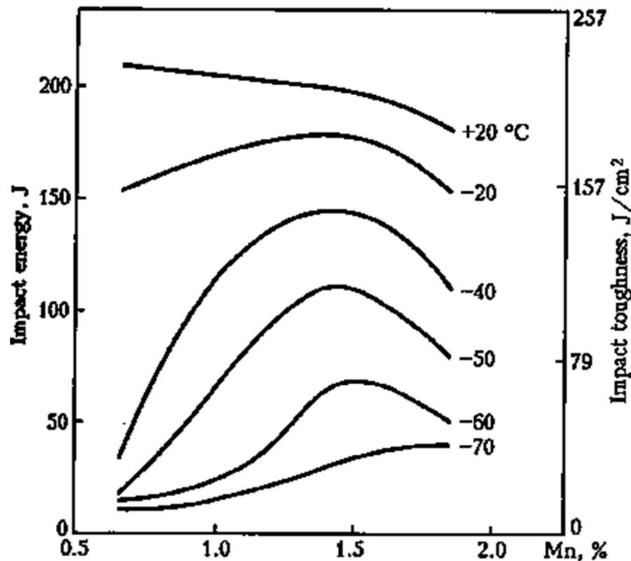
**Figure 3.2.1:** Influence of manganese content on impact energy and impact toughness of weld metal at different temperature [58]
