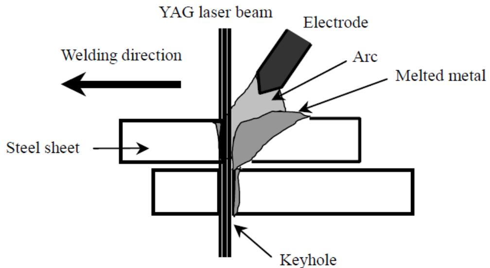
**Figure 2.3.6:** A typical hybrid laser-arc welding [43]
