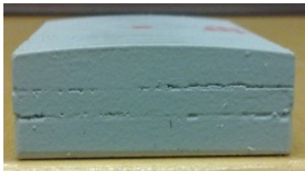
Fig. 3.10. Three-layer magnet module of the MM machine. The top and bottom layers are made of a Ne493a grade magnet material. The material of the middle layer is a Somaloy 550 composite. The whole assembly is epoxy coated. The slitting of the topmost magnet is not shown because of the epoxy coating.
